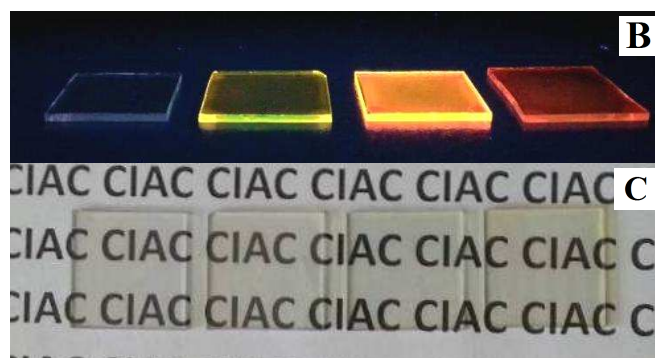
21 Figure 7. (A) A series of transmittance spectra, excitation spectra, and PL spectra of 22 bifacial ITO/glass/Cu-doped Zn_xCd_{1-x}S luminescent thin films with different Zn/Cd
