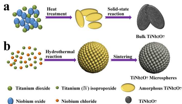
Scheme 1. Schematic comparison of growth process. (a) Conventional solid-state process for microsized bulk \text{TiNb}_2\text{O}_7 . (b) Novel one step solvothermal synthesis of hierarchical \text{TiNb}_2\text{O}_7 microspheres.
