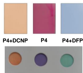
Figure 3. Silica gel plate (up) and polyethylene oxide membrane (down) of P4 in the presence of the DCNP and DFP vapours (30 ppm).
