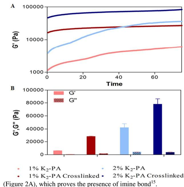
**Figure 3.** Rheological characterization of the gels. A) Gelation kinetics, B) Equilibrium moduli at pH 7.5.
