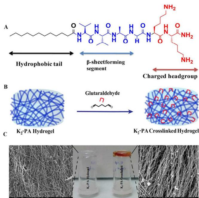
**Figure 1.** Schematic representation of peptide amphiphile chemical structure (A), peptide gel formation and glutaraldehyde crosslinking strategy (B), (C).
