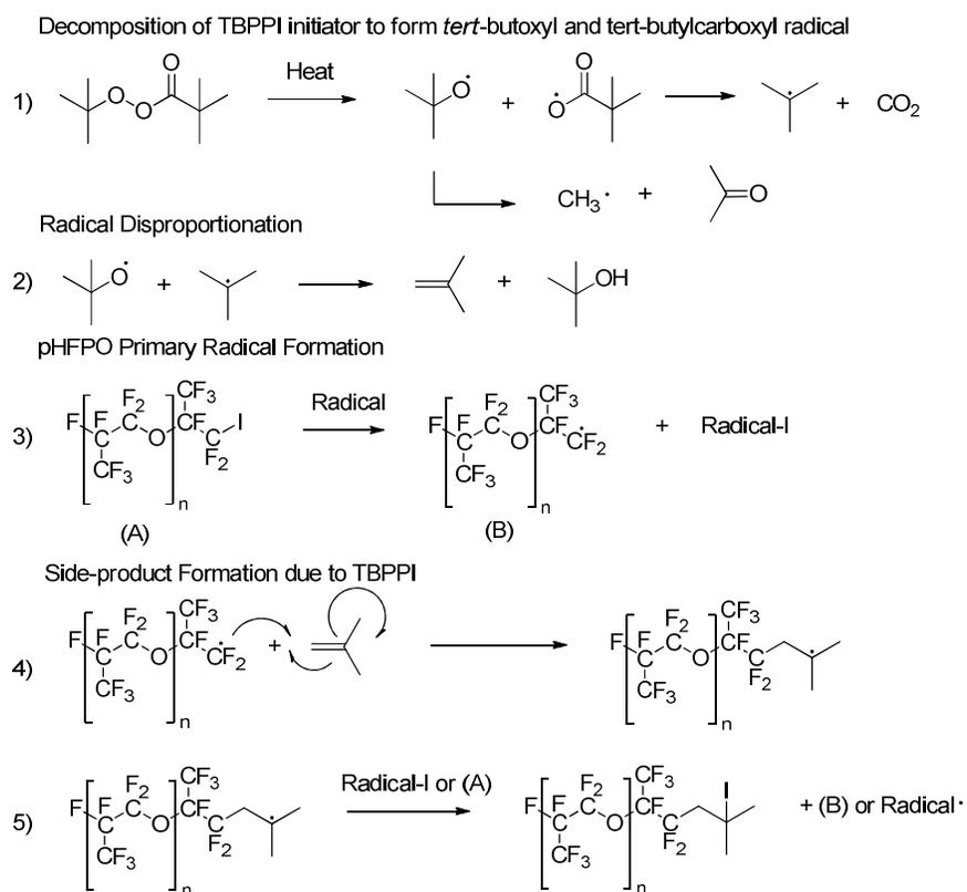
**Scheme 5. Conversion of poly(hexafluoropropylene oxide) primary iodide to undesired side-product using TBPPI as the radical initiator.**
