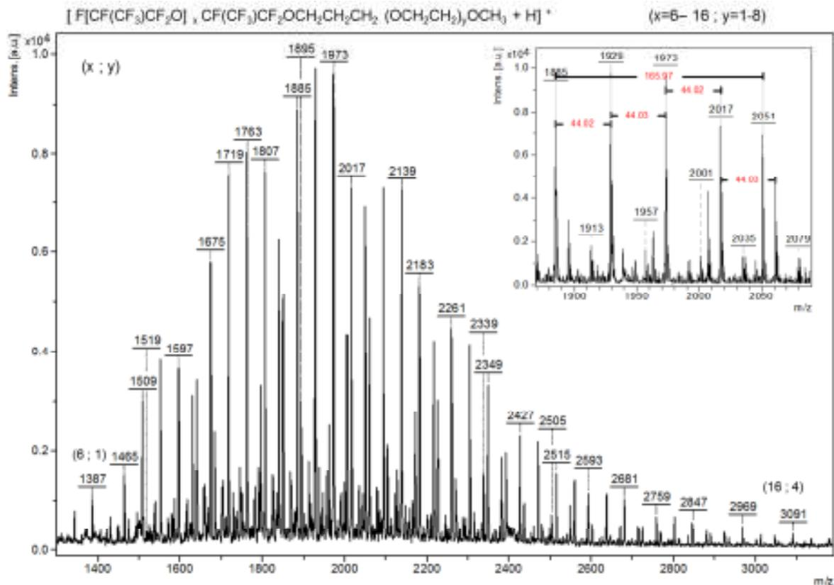
**Figure 6:** Positive ion mode MALDI-TOF-MS spectrum of oligo(HFPO)-CH<sub>2</sub>CH<sub>2</sub>CH<sub>2</sub>-oligo(PEG) (using as matrix DCTB and LiCl as the cationizing agent), 1807 m/z is x = 8 and y = 5. The insert expansion *m/z* between 1850 and 2100 displays 166 and 44 m/z-repeat units for HFPO [CF(CF<sub>3</sub>)CF<sub>2</sub>O] and ethylene oxide (CH<sub>2</sub>CH<sub>2</sub>O), respectively.
