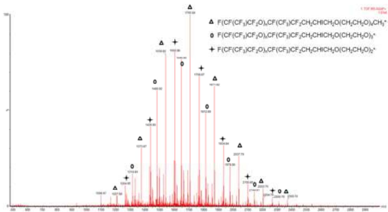
**Figure 5: Positive mode Atmospheric pressure Solids Analysis Probe (ASAP) time-of-flight mass spectrometry (TOF-MS) spectrum of  $F[CF(CF_3)CF_2O]_{8.9}CF(CF_3)CF_2CH_2CHICH_2O(CH_2CH_2O)_{9.5}-CH_3$  (initiated with BPO). 166 m/z is the repeat unit for HFPO  $[CF(CF_3)CF_2O]$  and 44 m/z is the repeat unit for ethylene oxide  $(CH_2CH_2O)$ .**
