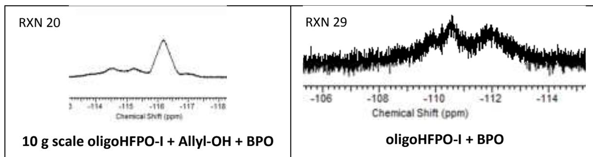
Figure 2: Comparison of the  $^{19}\text{F}$ -NMR expansions of  $^{19}\text{F}$  NMR spectra the reaction of oligo(HFPO)-CF(CF<sub>3</sub>)CF<sub>2</sub>I with the initiator (TBPPI, AIBN, BPO) (right column) and initiator with allyl alcohol (left column).
