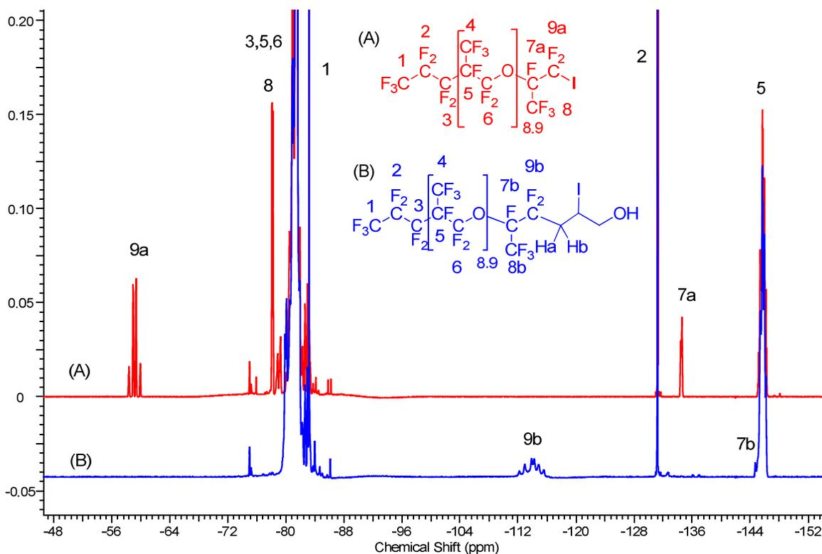
Figure 1:  $^{19}F$ -NMR spectra of 1-iodo-2-oligo(hexafluoropropylene oxide)perfluoropropane ( $F[CF(CF_3)CF_2O]_{8.9}CF(CF_3)CF_2I$ ) (A) and  $F[CF(CF_3)CF_2O]_{8.9}CH_2CHICH_2OH$  (B).
