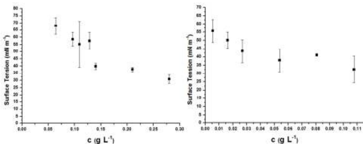
**Figure 7:** Surface tension measurements of new surfactant (Left) oligo(HFPO)-CH<sub>2</sub>CHICH<sub>2</sub>-oligo(PEG) [CMC = 0.13 g/L] (and Right) oligo(HFPO)-*b*-oligo(PEG)[CMC = 0.04 g/L]. Reference: APFO [CMC = 3.77 g/L] (Figure S42)
