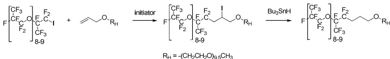
**Scheme 1.** Synthesis of oligo(hexafluoropropylene oxide)-*b*-polyethylene glycol, oligo(HFPO)-*b*-PEG diblock surfactant by radical addition of [oligo(HFPO)] primary iodide onto allyl PEG followed by a selective reduction of the iodine atom.
