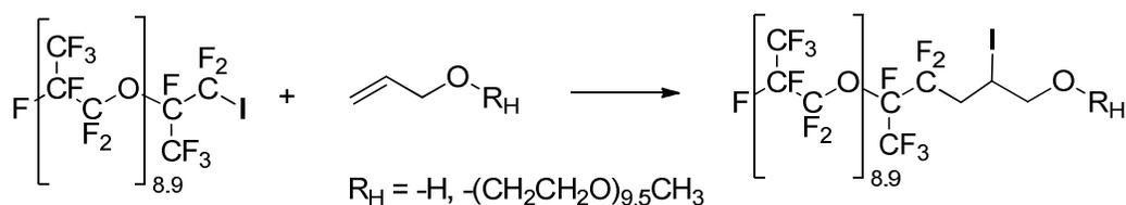
**Scheme 4. Radical reaction of 1-iodoperfluoropropyl-2-oligo(hexafluoro-propylene oxide) onto allyl alcohol and allyl-O-PEG-OCH<sub>3</sub> (initiated by AIBN, TBPPi, and BPO).**
