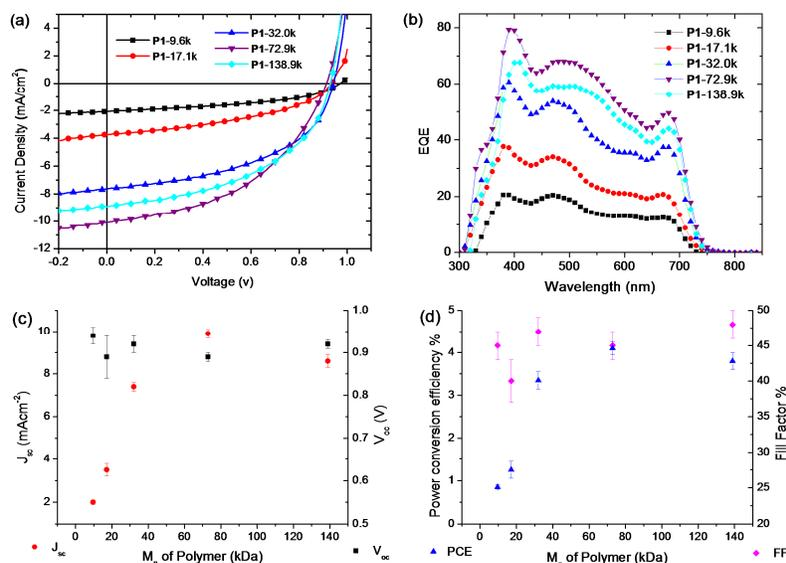
**Fig. 3** (a)  $J$ - $V$  characteristics of photovoltaic devices fabricated with different molecular weight **P1/PC<sub>71</sub>BM** under AM 1.5G irradiation ( $100 \text{ mW cm}^{-2}$ ). (b) EQE curves of the BHJ solar cells fabricated under the same optimized conditions as used for the  $J$ - $V$  measurements. (c)  $M_n$  of polymer plotted against  $J_{sc}$  and  $V_{oc}$  and (d)  $M_n$  of polymer plotted against FF and PCE.
