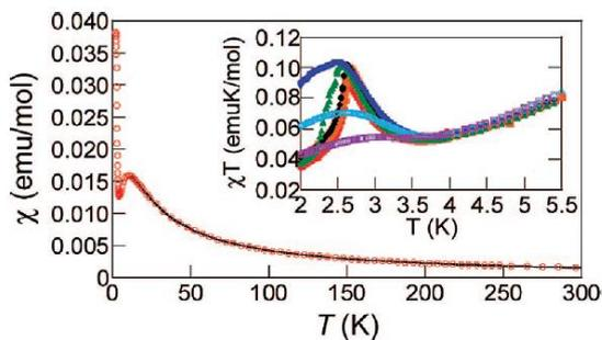
**Figure 3**  $\chi$  vs  $T$  plot for  $[\text{CuF}_2(\text{H}_2\text{O})_2(\text{pyz})]$ . The solid line represents the theoretical fit. Inset shows the  $\chi T$  vs  $T$  plot at different external field values (50 G = red, 100 G = orange, 250 G = black, 500 G = green, 1000 G = blue, 2500 G = cyan, 5000 G = purple). Reprinted with permission from ref. 5. Copyright 2008 American Chemical Society.
