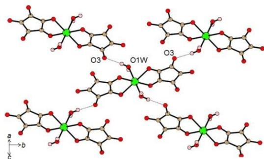
**Figure 5** Intralayer H-Bonds between discrete  $[Fe(C_5O_5)(H_2O)_2]^{2-}$  units. Colour codes: C = brown, O = red, H = pink, Fe = green. Reprinted with permission from ref. 8. Copyright 2012 American Chemical Society.
