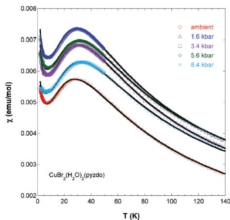
**Figure 8** Magnetic susceptibility for  $[CuBr_2(pyzo)(H_2O)_2]$  as a function of the applied pressure. Reprinted with permission from ref. 16. Copyright 2012 American Chemical Society.
