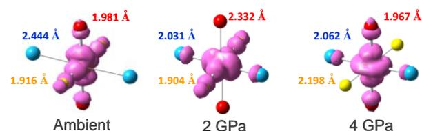
**Figure 4** Schematic illustrating the pressure-induced reorientation of the magnetic orbitals in  $[\text{CuF}_2(\text{H}_2\text{O})_2(\text{pyz})]$ . Color codes: F = yellow, O = red, N = cyan.
