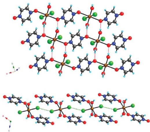
**Figure 6** View of the crystal structure of  $[CuBr_2(pyzo)(H_2O)_2]$  where the intermolecular interactions between the chains are highlighted (top: H-bonding; down: halogen bonding). Adapted with permission from ref. 16. Copyright 2012 American Chemical Society.
