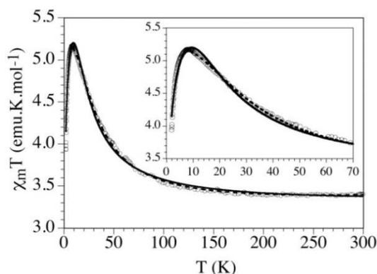
**Figure 6** Thermal variation of the  $\chi T$  for  $K_4[Fe(C_5O_5)(H_2O)_2](HC_5O_5)_2 \cdot 4H_2O$ . Solid and dashed lines show the best fit of the employed models. Reprinted with permission from ref. 8. Copyright 2012 American Chemical Society.
