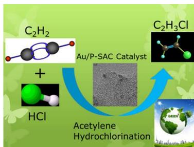
Text: gold-based catalysts supported on Phosphorus-doped carbon are used in acetylene hydrochlorination to enhance the catalyst activity.
