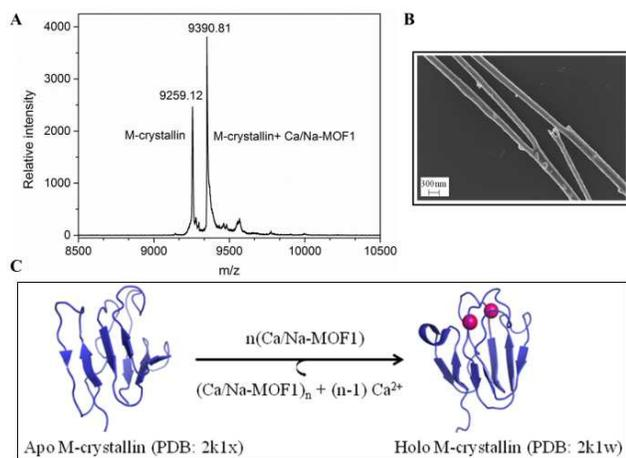
Figure 4. (A) Representative MALDI-TOF mass spectrum of M-crystallin titration with Ca/Na-1 at 1:2 ratio of protein vs Ca/Na-1. (B) FE-SEM image of Ca/Na-1 after  $\text{Ca}^{2+}$  release. (C) Schematic showing  $\text{Ca}^{2+}$  release from Ca/Na-1 and conversion of apo M-crystallin to holo form.
