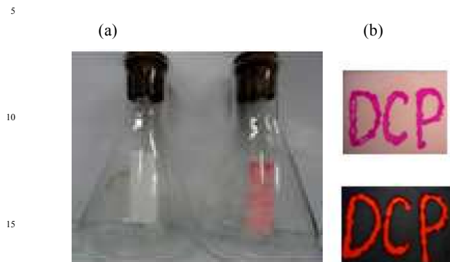
Figure 8: (a) Change of TLC plate (coated with RHM) in presence of DCP vapour and (b) Change of TLC plate (coated with RHM) in presence of DCP solution in sunlight (up) and under UV-light (below).
