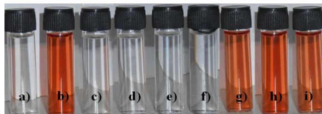
Fig. 1 Visual color change of L ( 1 \times 10^{-5} M) in dry CH 3 CN after the addition of 2 equivalents of TBA salts. a) Free receptor L , b) F - , c) Cl - , d) Br - , e) I - , f) H 2 PO 4 - , g) CH 3 COO - , h) mixture + F - and i) mixture + CH 3 COO - .
