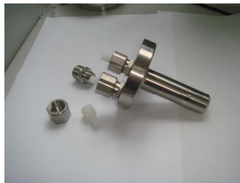
Fig.4 Test pins mounted by setscrews with rigid sample holders
