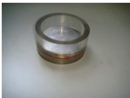
Fig.3 Lubricant brim consisting of the test disk, PVC brim and O-ring seal
