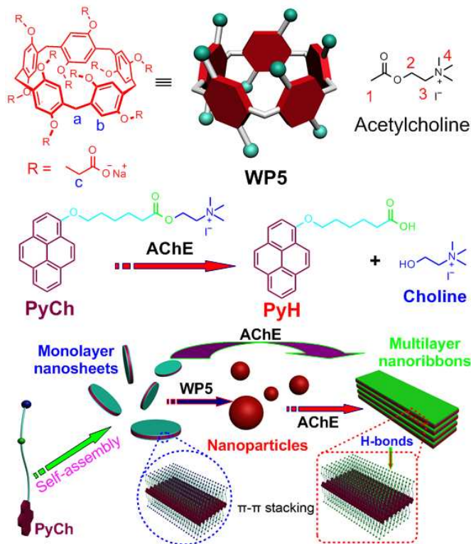
Fig. 1 Structural illustration of the building blocks ( WP5 , PyCh and acetylcholine) and schematic representation of the resulting enzyme-responsive self-assembly.
