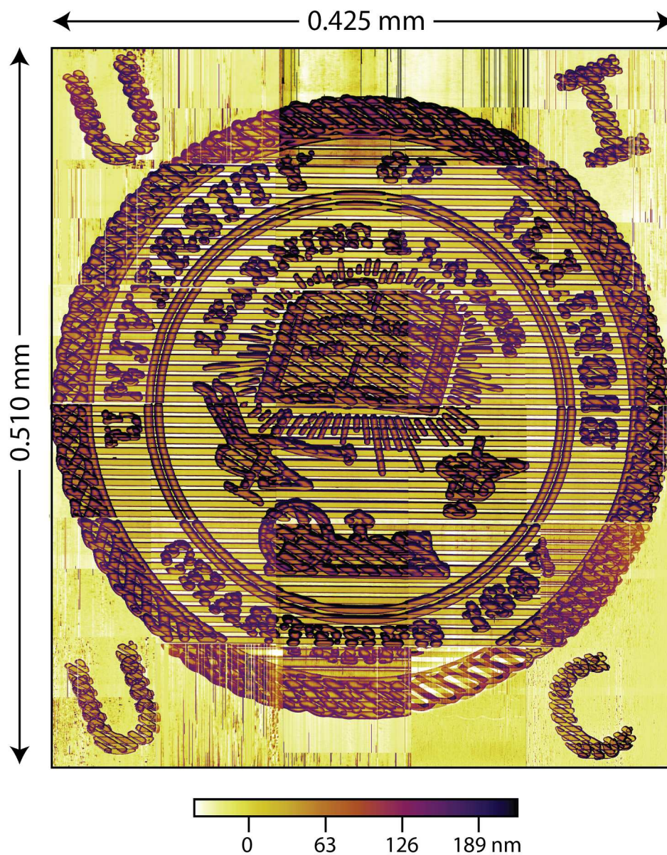
Figure 7: A 0.510 mm × 0.425 mm composite AFM image consisting of 9.05 million pixels, acquired simultaneously with 30 cantilevers. The array scanned the substrate in contact-mode AFM at 226 \mu\text{m}/\text{sec} and the image was acquired in 256 seconds. Each cantilever scanned a 90 \mu\text{m} × 90 \mu\text{m} area and the resulting 30 scans were stitched to make the complete image. 536x676mm (96 x 96 DPI)
