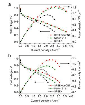
**Fig. 3** Single cell performance of membrane-electrode-assembly (MEA) 95 with SPEEK/dsCNT, SPEEK and Nafion 212 membranes at 100% RH and (a) 75 °C and (b) 90 °C.
