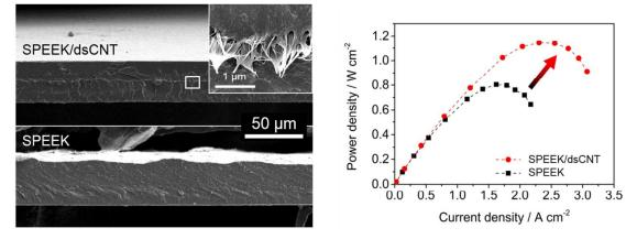
Text: A composite proton exchange membrane prepared by electrospinning SPEEK and direct spinning of CNTs is more robust than SPEEK alone and outperforms SPEEK and Nafion 212 membranes.
