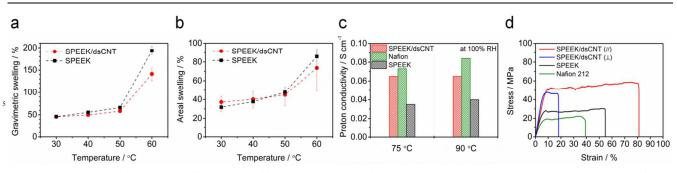
Fig. 2 (a) Gravimetric and (b) areal swelling of SPEEK/dsCNT and SPEEK, and the (c) proton conductivity and (d) stress-strain of SPEEK/dsCNT (parallel and perpendicular to the dsCNT web layer), SPEEK and Nafion membranes.
