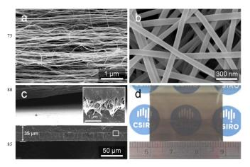
Fig. 1 SEM images of the (a) dsCNT web, (b) electrospun SPEEK (c) cross-section of SPEEK/dsCNT membrane, with inset image showing higher magnification and optical image (d) of the SPEEK/dsCNT <sup>90</sup> membrane.
