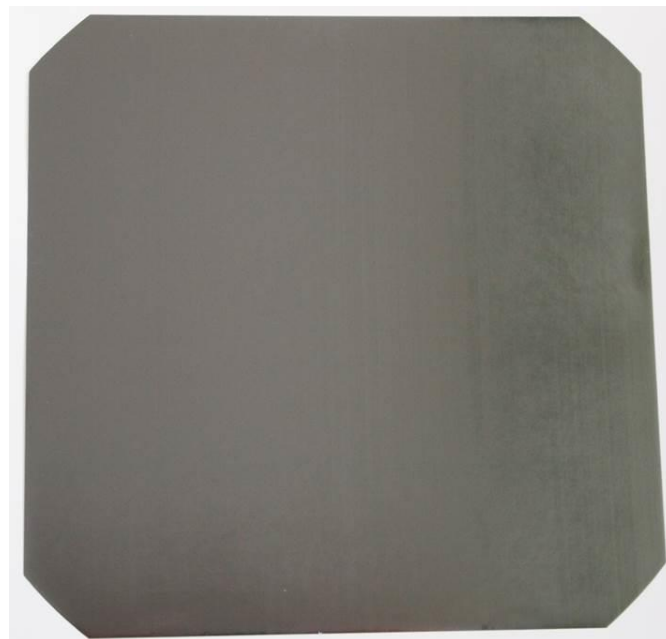
Fig. 9 Image of a recycled wafer obtained by etching process #2.
