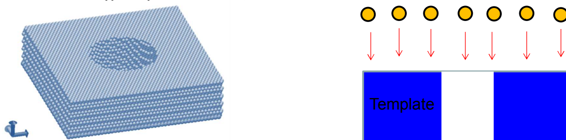
Fig. 9 (a) Copper template with (111) on surface and a hole in the center, and (b) deposit of carbon atoms placed at 0.5 nm above the Cu (111) surface for the growth of 3D CNT-graphene nanostructures.
