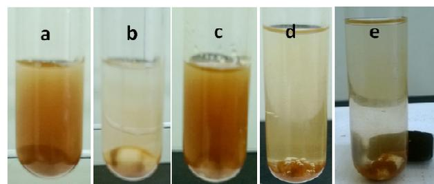
Fig. 13 Photo of a: Fe(ox)-Fe<sub>3</sub>O<sub>4</sub> nanoparticle in water; b: Fe(ox)-Fe<sub>3</sub>O<sub>4</sub> nanoparticle adsorbed on the magnetic stirring bar; c: Fe(ox)-Fe<sub>3</sub>O<sub>4</sub> nanoparticle in the reaction mixture; d: after the completion of reaction in acetone-water; e: a magnet attract the Fe(ox)-Fe<sub>3</sub>O<sub>4</sub> nanoparticle and magnetic stirring bar.
