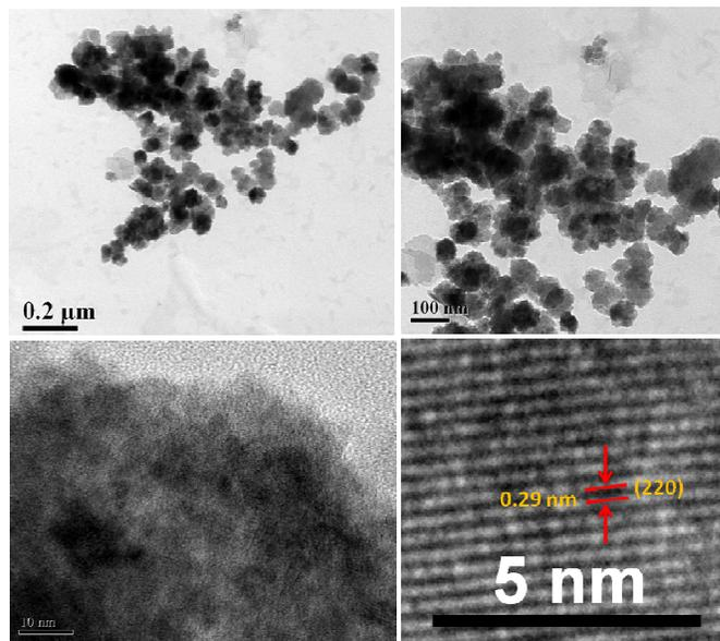
Fig. 11 TEM/HR-TEM image of  $\text{Fe}_3\text{O}_4$ .
