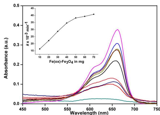
Fig. 17 Fe(ox)-Fe<sub>3</sub>O<sub>4</sub> promoted photo degradation of methylene blue under UV-light and the effect of catalyst on photodegradation rate.
