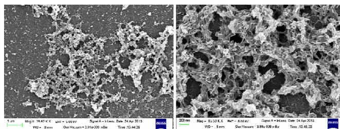
Fig. 10 HR-SEM image of  $\text{Fe}(\text{ox})\text{-Fe}_3\text{O}_4$ .
