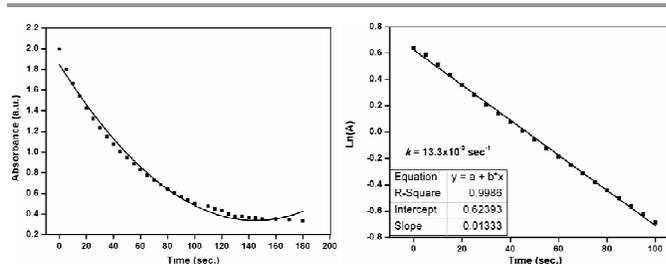
Fig. 6 Rate kinetics of Fe(ox)-Fe(0) catalyzed reduction of methylene blue.
