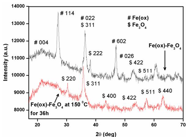
Fig. 8 XRD pattern of  $\text{Fe}(\text{ox})\text{-Fe}_3\text{O}_4$  and its decomposed product  $\text{Fe}_3\text{O}_4$ .
