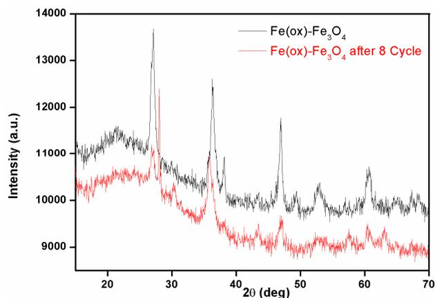
Fig. 15 XRD pattern of Fe(ox)-Fe<sub>3</sub>O<sub>4</sub> before and after the completion of 8 cycle.
