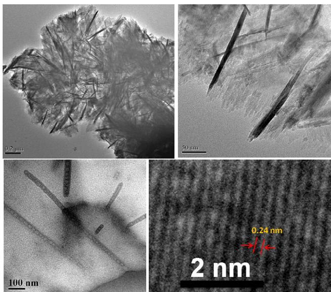
Fig. 9 TEM/HR-TEM image of  $\text{Fe}(\text{ox})\text{-Fe}_3\text{O}_4$ .
