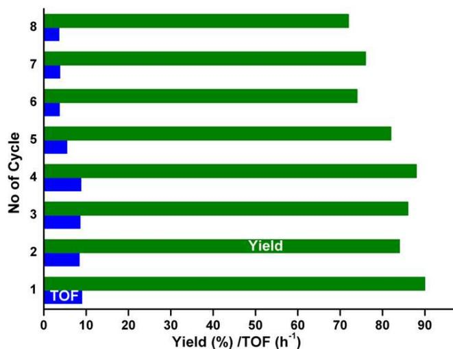
Fig. 14 catalytic cycle vs turn over frequency (TOF) and yield plot of Fe(ox)-Fe<sub>3</sub>O<sub>4</sub> catalyzed condensation reaction between 4-bromo benzaldehyde and indole.
