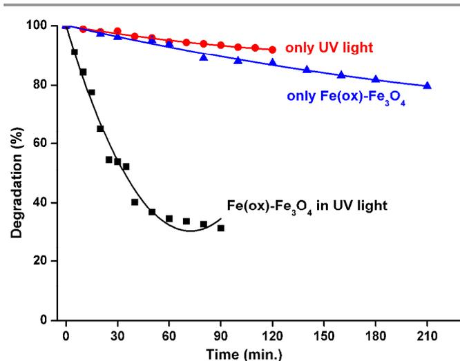
Fig. 16 Fe(ox)-Fe<sub>3</sub>O<sub>4</sub> promoted photo degradation of methylene blue under different environment.
