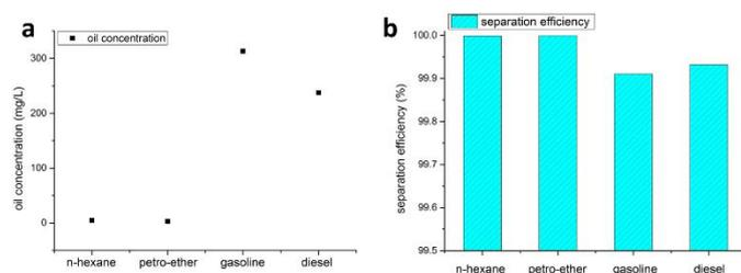
**Fig. 4** a) The oil concentration of water samples after separation, in which different kinds of oil/water mixture were used (hexane/water, petro-ether/water, gasoline/water and diesel/water). b) The separation efficiency calculated with the equation:  $E = 1 - C/C_0$ ,  $E$  for the separation efficiency,  $C$  for the oil concentration in the water samples after separation and  $C_0$  for the equivalent oil concentration of the mixture before separation.
