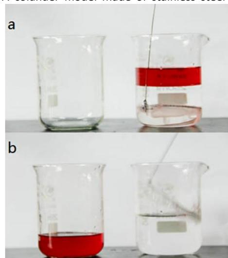
cellulose-coated mesh, which could scoop oil (n-hexane dyed by oil red) from water. b) After several times of scooping, oil/water mixture was separated and oil was collected to the other beaker with imperceptible amount of water inside.
