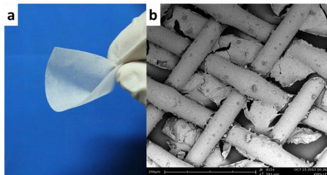
**Fig.1** a) A macro view of the as prepared cellulose-coated nylon mesh, which is very soft. b) Typical SEM image of cellulose-coated nylon mesh. The surface of nylon fibre was covered by cellulose hydrogel and the pores were left unblocked.
