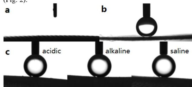
**Fig. 2.** Contact angle of the cellulose hydrogel coated mesh. The mesh is a) superhydrophilic in air with WCA of  $0^\circ$  and b) superoleophobic underwater with OCA above  $150^\circ$ . 1, 2-dichloroethane was used as oil droplet. c) The mesh could sustain superoleophobicity in alkaline (0.1 mol/L sodium hydroxide), acidic (0.1 mol/L muriatic acid) and saline aqueous (1 mol/L sodium chloride) phases.
