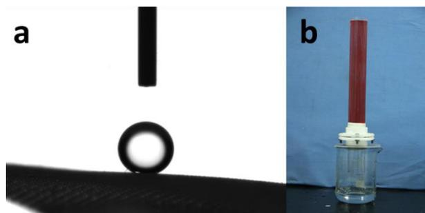
**Fig.6** a) the mesh could maintain its underwater superoleophobicity after 12 times of cycling use and kept in water for 90 days. The oil droplet is 1,2-dichloroethane, and the oil contact angle is  $154^\circ$ . b) After oil/water separation, the mesh could sustain 110mL n-hexane (dyed with oil red) upside. The oil's height is 19.5cm and the pressure on the mesh is 1260Pa.
