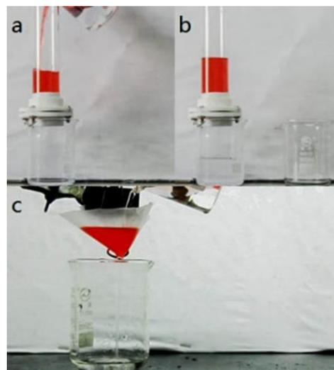
**Fig. 3** a) The device for oil/water separation consists of a glass tube, a PTFE clamp and a 100 mL beaker. The mesh was fixed by the clamp and 60 mL oil/water mixture (n-hexane : water=1:1, v/v) was poured into the glass tube. b) After the separation, oil was sustained upside and water passed through the mesh to the beaker. c) A clear view during the separation. Water passed the mesh instantaneously while oil (n-hexane dyed by oil red) was blocked upside.
