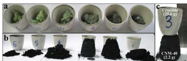
Fig. 5 Photographs of (a) PP/OMMT-NiO- x (5.2–5.5 g) in the crucible (30 mL), (b) CNMs from PP/OMMT-NiO- x after being removed off the crucible, and (c) the crucible (25.6 g) supported by sponge-like CNM-40 (2.2 g). Crucible 1 # was marked for PP/OMMT-NiO-400 or CNM-18, crucible 2 # for PP/OMMT-NiO-500 or CNM-26, crucible 3 # for PP/OMMT-NiO-600 or CNM-40, crucible 4 # for PP/OMMT-NiO-700 or CNM-96, crucible 5 # for PP/OMMT-NiO-800 or CNM-128, and crucible 6 # for PP/OMMT-NiO-900 or CNM-227.
