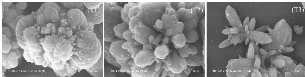
Fig. 6 (T1), (T2) and (T3) are representative SEM images of the TiO 2 flowers obtained at different cooling conditions after heating up to 180 °C for 2 hrs.
