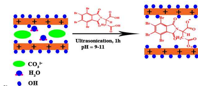
Figure 1. Intercalation of diacid in the interlayer of LDH
