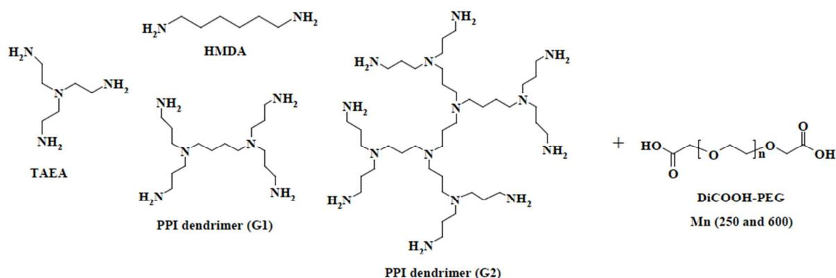
**Figure 1.** Amines and carboxylic acid end-functionalised PEGs creating the supramolecular ionic structures.
