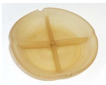
Figure 9: Sample of starch plasticised with glycerol and choline chloride injection moulded into a 10 cm mould (200 °C and 60 bar). Sample diameter 7 cm.
