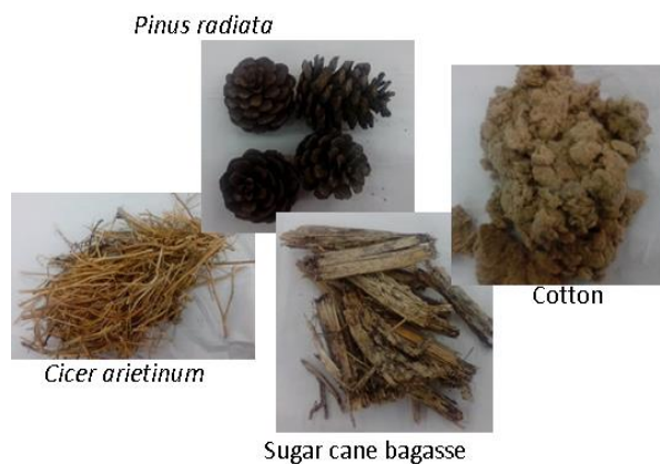
Fig. 1. Cellulosic feedstocks used for levulinic acid production
