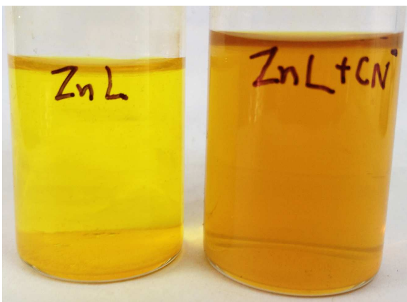
Figure 9. Naked eye determination of cyanide ion in aqueous sample using (ZnL)
