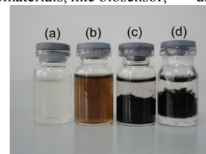
Figure 1. Microbial reduction of GO and biosynthesis of N-graphene occurred under anaerobic conditions. (Serum bottles a=pure denitrifying bacteria in the denitrifying medium without GO; b=blank control without bacteria; c=denitrifying bacteria microbial-reduced graphene (DNMG)-1 with bacteria after 3 days; d=DNMG-2 with bacteria after 5 days.)
