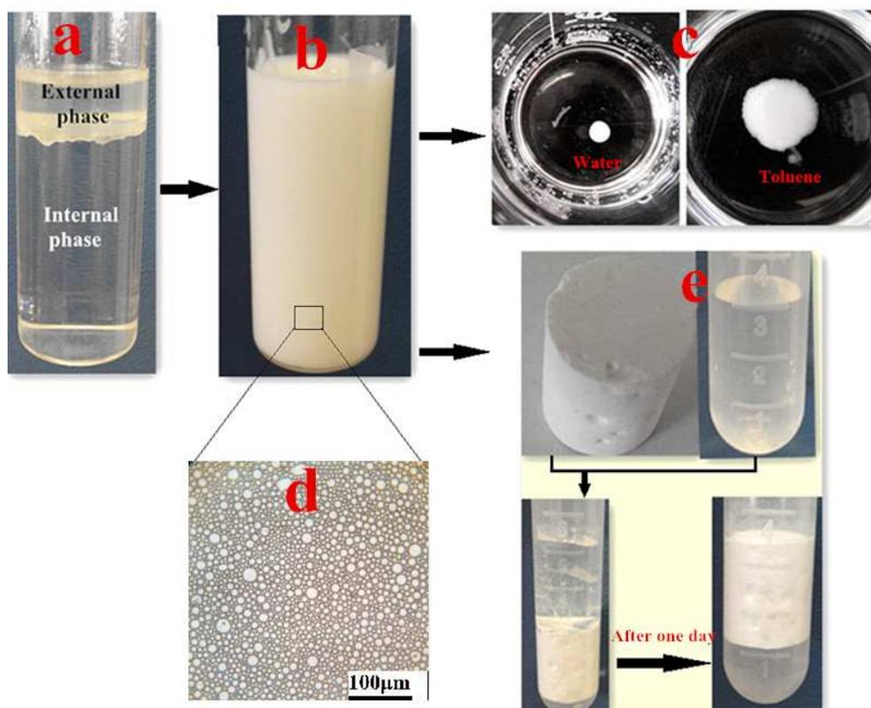
Fig. 2 Exposition of prepared Pickering W/O HIPEs and PDVB-SS-X-SO<sub>3</sub>H using the experimental progress of PDVB-SS-0.2-SO<sub>3</sub>H (a) phase-separated system, (b) Pickering W/O HIPEs with an 84.8 vol % internal phase fraction, (c) the Pickering W/O HIPEs dispersed in water and toluene, respectively, (d) micrograph of the Pickering W/O HIPEs, (e) PDVB-SS-0.2-SO<sub>3</sub>H monolith soaked in water.
