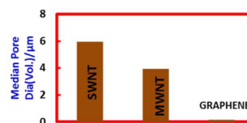
Figure 2. Porometric data for NAM with graphene, SWNT and MWNT additives
