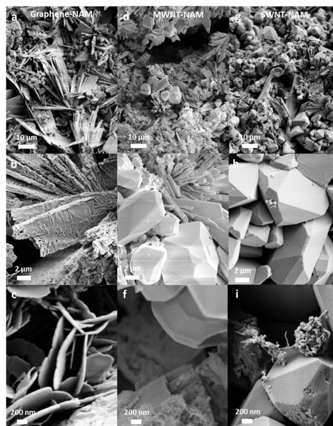
Figure 4. FE-SEM image of cycled NAM (after cell failure) with (a,b,c) Graphene, (d,e,f) MWNT and (g,h,i) SWNT.
