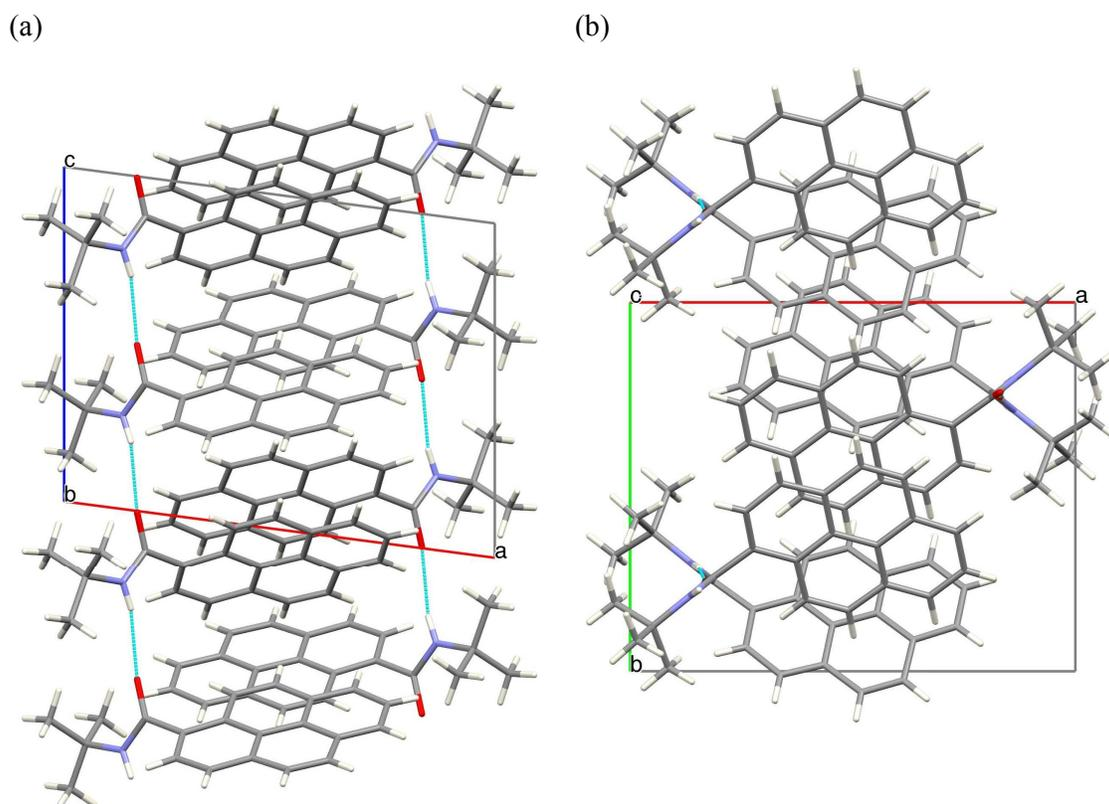
Figure 9. Crystal packing of **2c** viewed along the crystallographic (a) b-axis (b) c-axis. H-bonds marked in cyan.
