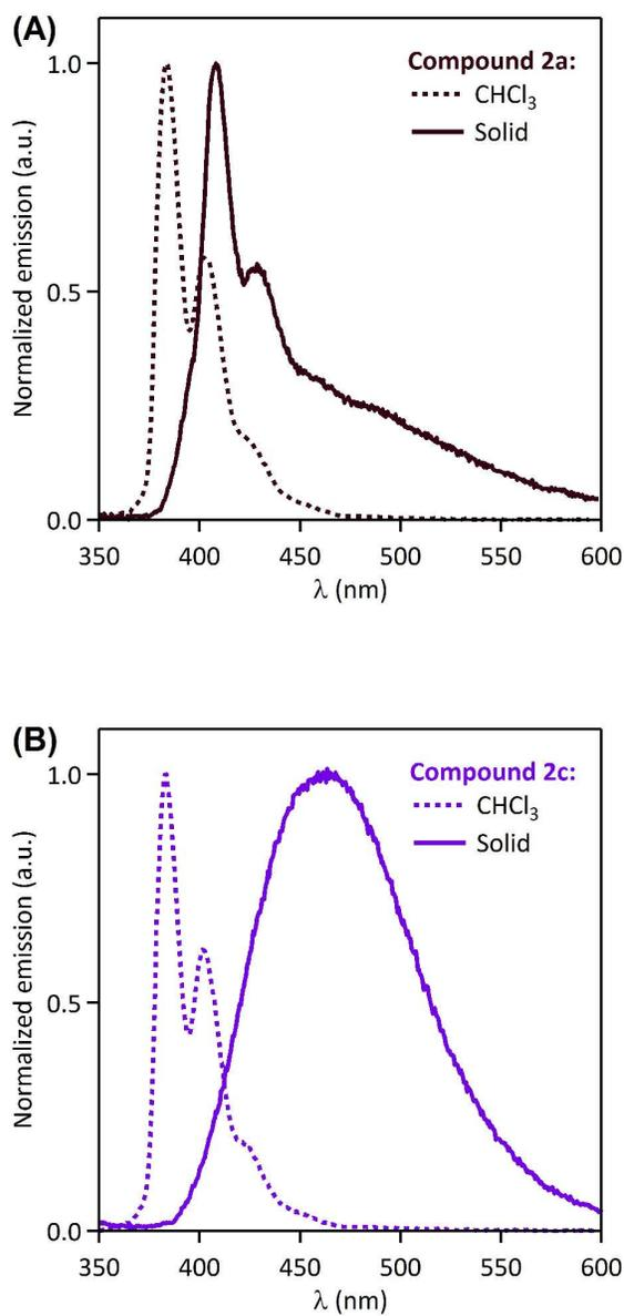
Figure 2. Normalized solution (CHCl<sub>3</sub>) and solid-state fluorescence emission spectra of **2a** (A) and **2c** (B).
