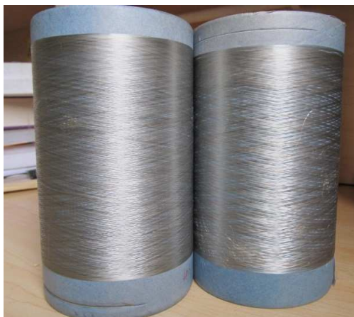
Fig. 1 Picture of a several hundred meters long PVA/rGO composite fiber on the wheels.
