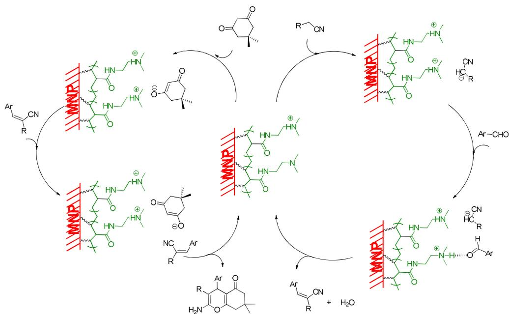
**Scheme 2.** Plausible mechanism for synthesis of product through basic site of catalyst
