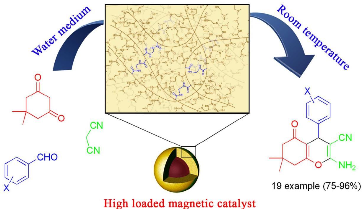
A high loaded basic magnetic catalyst was synthesized by distillation-precipitation-polymerization method. The catalyst shows high activity in water medium for the synthesis of 4*H*-benzopyrans.
