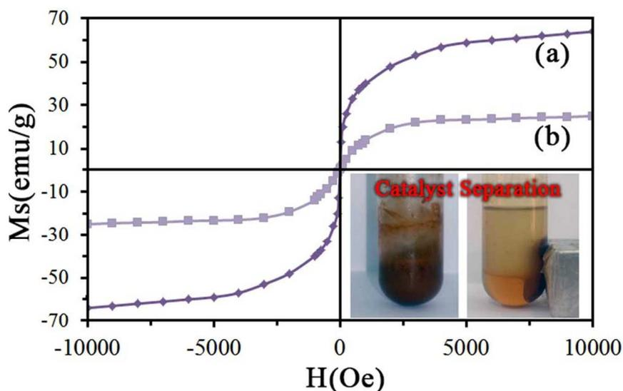
**Fig. 3.** VSM curves for  $\text{Fe}_3\text{O}_4$  (a),  $\text{MNP@PDMA}$  (b) and magnetic recovery of catalyst (inserted image)
