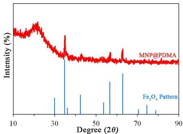
**Fig. 2.** XRD diffraction patterns of the catalyst MNP@PDMA
