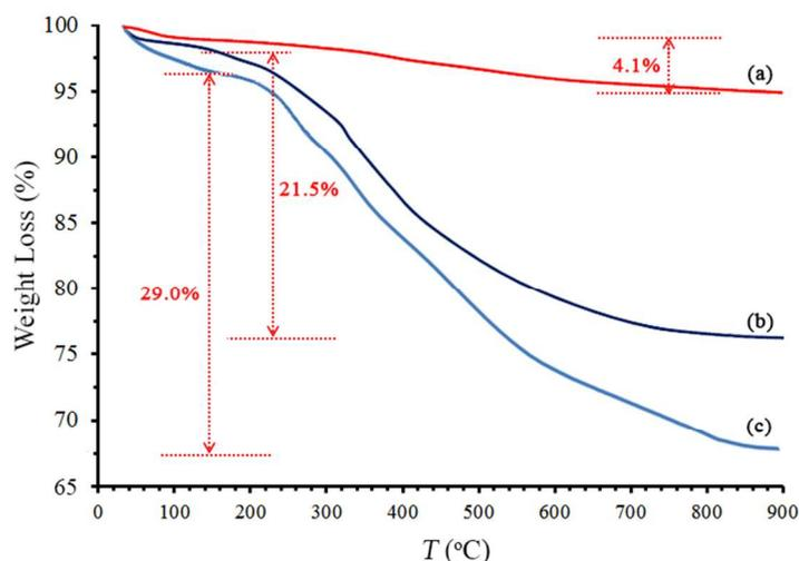
**Fig. 4.** TGA carves of (a) MNP@MPS, (b) MNP@PMA, and (c) MNP@PDMA
