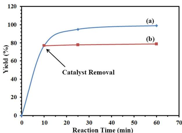
**Fig. 7.** Leaching experiment. (a) reaction in the presence of catalyst and (b) reaction after removal of catalyst.
