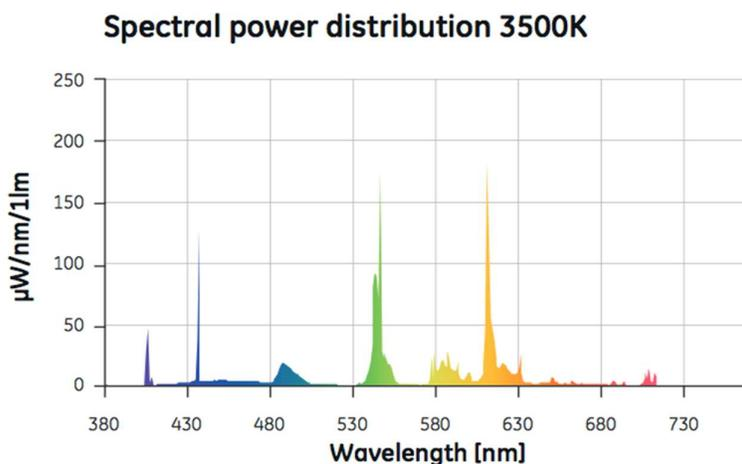
Figure 4: Spectral Power Distribution of General Electric 28W Miser™ 2D lamp.<sup>16</sup>
