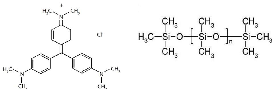
Figure 1: Chemical structures of (left) the photosensitizer dye, crystal violet, and the silicone elastomer polydimethylsiloxane.<sup>13, 14</sup>
