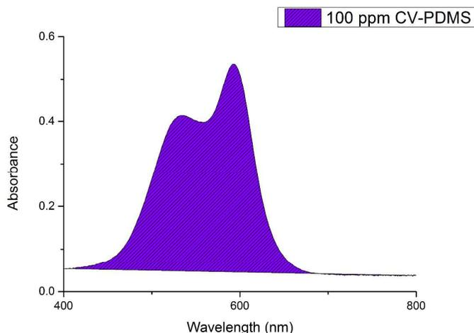
Figure 3: UV-vis absorbance spectra of CV-coated silicon polymer at a concentration of 100 ppm
