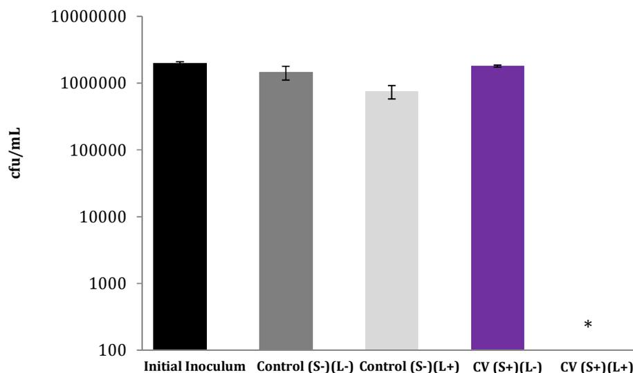
Figure 6: Numbers of *E. coli* on the surfaces of the polymers after 6 h exposure. Bars on the graph represent the: initial inoculum, control elastomer (control) and CV-encapsulated elastomer (CV). (L+ = white light exposure, L- = no white light exposure, S+ = CV dye present, S- = CV dye not present). The asterisk indicates where the bacterial numbers are below the detection limit of 100 cfu/mL.
