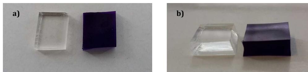
Figure 2: Images of PDMS samples a) before -on the left- and after the swell-encapsulation-shrink process in chloroform with 1000 ppm of crystal violet -on the right. (b) A cross section of the polymers prepared by immersion in 1000 ppm crystal violet dipping solution for 72 h.
