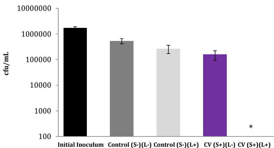
Figure 7: Numbers of *S. aureus* on the surfaces of the polymers after 2 h exposure. Bars on the graph represent the: initial inoculum, control elastomer (control) and CV-encapsulated elastomer (CV). (L+ = white light exposure, L- = no white light exposure, S+ = CV dye present, S- = CV dye not present). The asterisk indicates where the bacterial numbers are below the detection limit of 100 cfu/mL.
