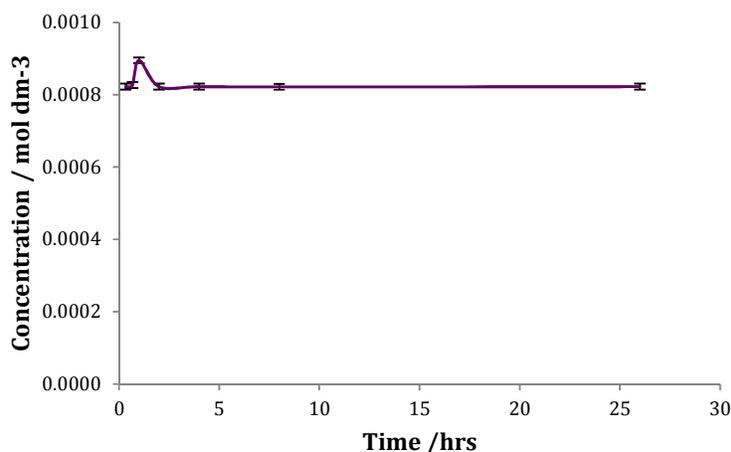
Figure 5: Leaching of crystal violet ( $\text{mol dm}^{-3}$ ) from a CV-coated silicon polymer into PBS solution at 37  $^{\circ}\text{C}$ , was measured as function of time (hours).
