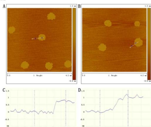
**Figure 2.** AFM images and height profiles of RGO (A, C) and GH (B, D).
