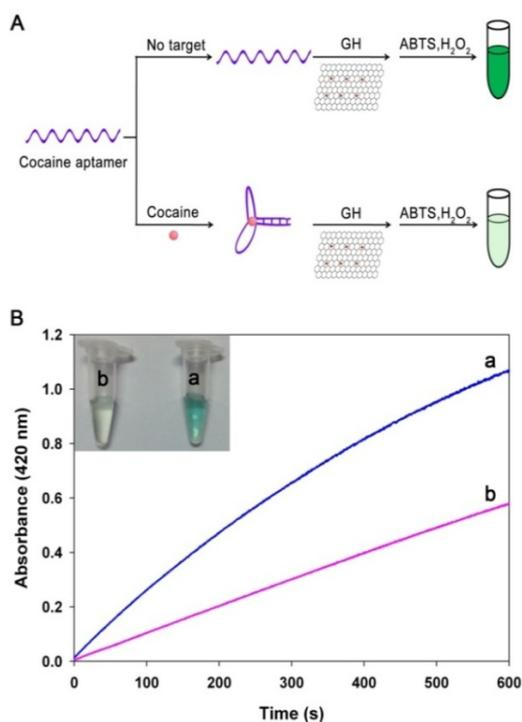
**Figure 5.** A) Schematic illustration of procedures for cocaine detection. B) Time-dependent absorbance changes at 420 nm in the absence of cocaine (a) and in the presence of cocaine (b, 50 mM).
