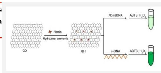
A novel colorimetric platform has been developed for detecting DNA and small molecule based on graphene–hemin hybrid nanosheet in homogenous solution.
