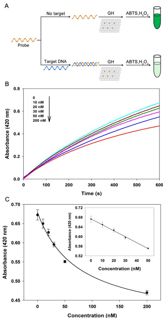
**Figure 4.** A) Schematic illustration of procedures for DNA detection. B) Time-dependent absorbance changes at 420 nm in the presence of different amounts of target DNA (0, 10, 20, 30, 50, 200 nM). C) Calibration curve corresponding to the absorbance for varying concentrations of target DNA with an intervening time of 10 min. Inset shows a linear calibration curve from 10 to 50 nM. The error bars represent the standard deviation of three experiments.
