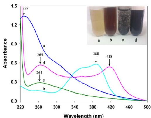
**Figure 1.** UV-Vis spectra of GO suspension(a), hemin solution (b), RGO suspension (c) and GHs suspension (d). Inset: photographs of GO (0.5 mg/mL) (a), hemin (0.5 mg/mL) (b), RGO (0.25 mg/mL) (c) and GHs (200  $\mu\text{g/mL}$ ) (d).
