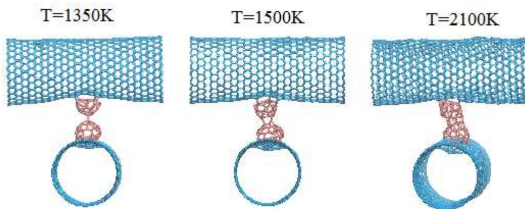
**Figure 2:** Heat-welded junction formed by CNT pairs (26, 0) with nanobuds at different temperatures 1350K, 1500K and 2100K
