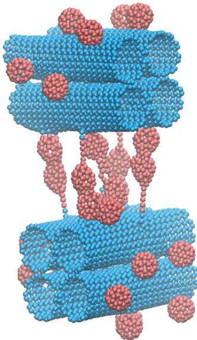
**Figure 5:** A typical simulation slide in the tensile process when separating the two SWCNTs bundles with junction via nanobuds
