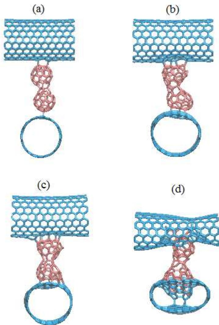
**Figure 1:** Typical heat-welded junction formed by nanobudes at temperature 1900K
