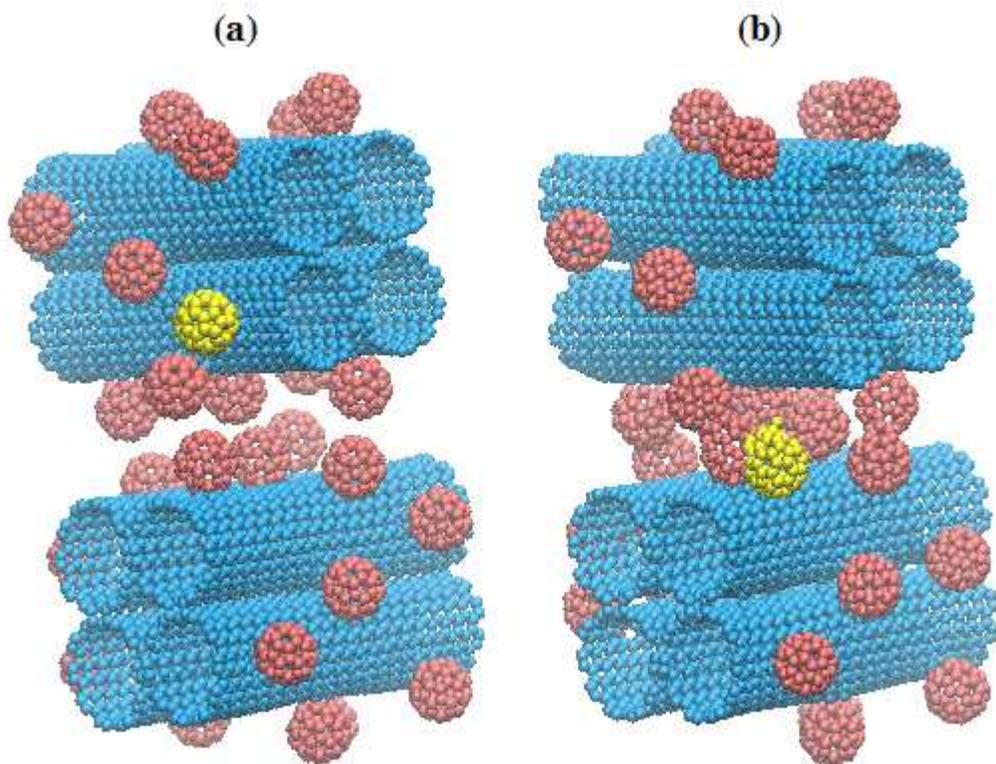
**Figure 4:** Heat welded carbon nanotube bundles via nanobuds: (a) two crossed SWCNTs bundles with nanobuds before heat welding. (b) two crossed SWCNTs bundles with junction formed after heat welding via nanobuds.
