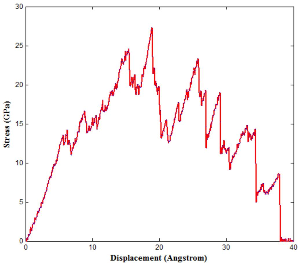
**Figure 6:** The tensile stress versus displacement relationships when separating the two SWCNTs bundles with junction via nanobuds
