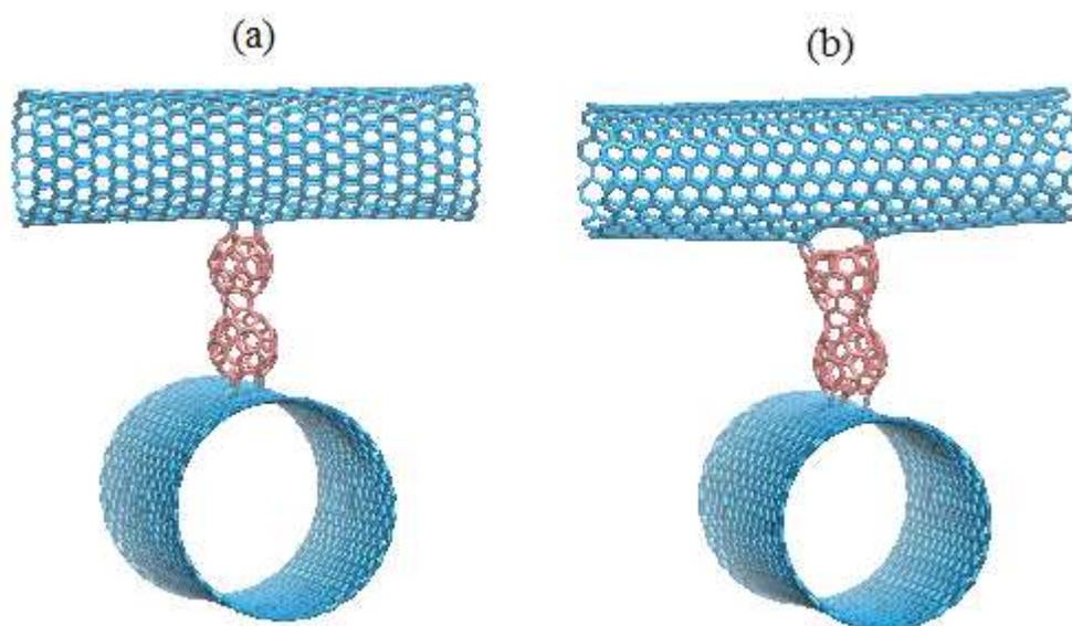
**Figure 3:** Heat-welded junction formed by two SWCNTs of different diameter and chiralities with nanobuds at temperature 1500K: (a) heat welded junctions of SWCNT pairs (18, 0)-(30, 0); (b) heat welded junctions of SWCNT pairs (10, 10)-(26, 0).
