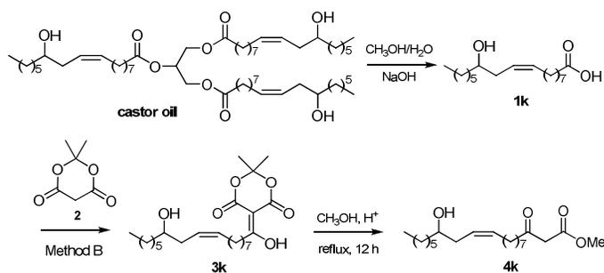
**Scheme 4** Synthesis of a fatty  $\beta$ -ketoester from Meldrum's acid (**2**) and ricinoleic acid (**1k**, Method B).
