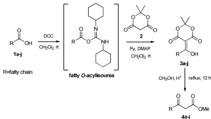
**Scheme 3** Synthesis of fatty  $\beta$ -ketoesters **4a-j** from Meldrum's acid (**2**) and the fatty acids **1a-j** (Method B).
