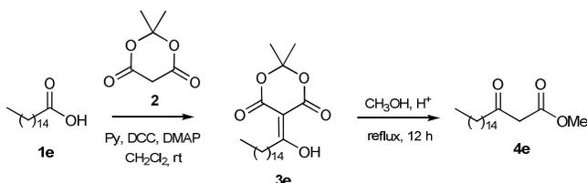
**Scheme 2** Synthesis of fatty  $\beta$ -ketoester **4e** from Meldrum's acid (**2**) and fatty acid **1e** using DMAP and DCC as the coupling agents (Method A).
