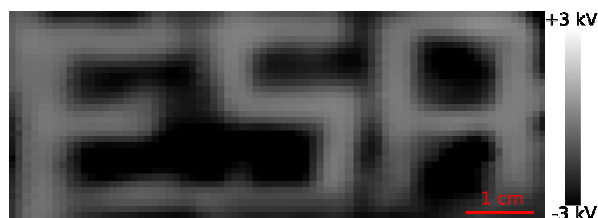
Fig. 16 Electrostatic lithography on a previously tribocharged PTFE sheet.
