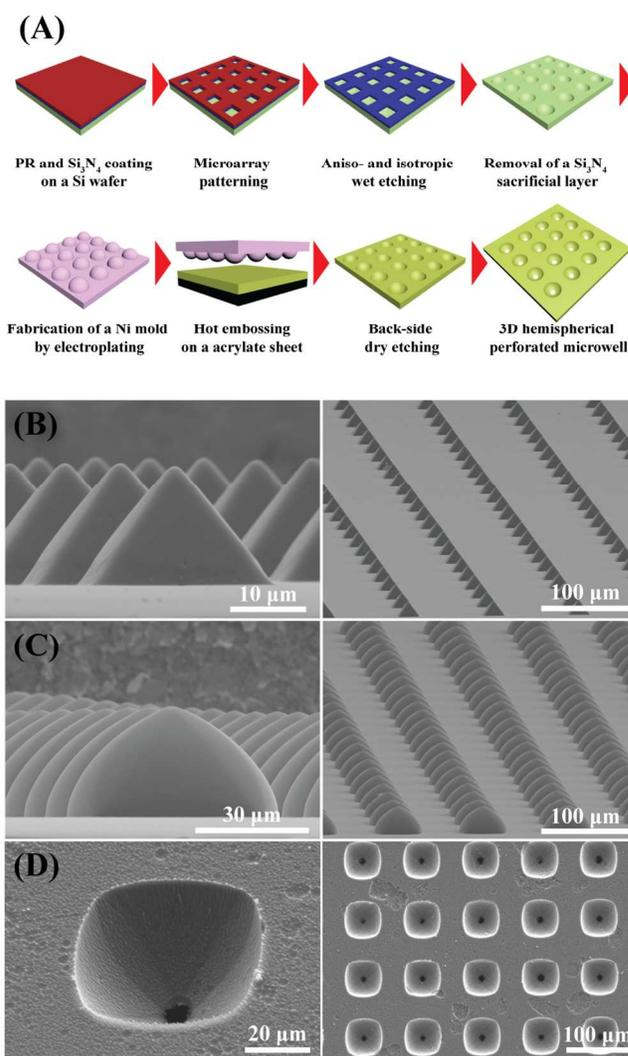
**Fig. 1** (A) Fabrication process of hemispherical perforated microwell structure. SEM images of a replicated PDMS from a Si wafer (B) after anisotropic wet etching and (C) aniso- and isotropic wet etching. (D) SEM image of a large-scale hemispherical perforated microwell structure.
