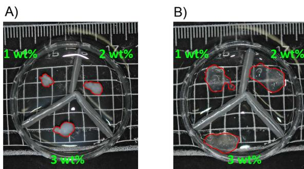
**Fig. 2** PAU hydrogels at 6 °C (A) and 34 °C (B) cross-linked by glutaraldehyde (1 – 3 wt%) in 10 mM HEPES (pH 7.5) containing 150 mM NaCl. Red lines trace gel edges.
