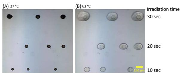
**Fig. 4** PAU gels at 27 °C (A) and 63 °C (B) prepared by UV irradiation (10 – 30 sec) 10 mM HEPES (pH 7.5) containing 150 mM NaCl.
