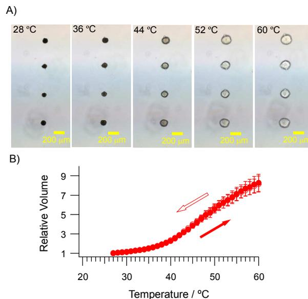
**Fig. 3** Volume transition of photocrosslinked microgels composed of AP-PAU in 10 mM HEPES (pH 7.5), 150 mM NaCl. (A) Microgels at various temperatures. (B) Relative volumes of microgels as a function of temperature during heating (closed circles) and cooling (opened circles).
