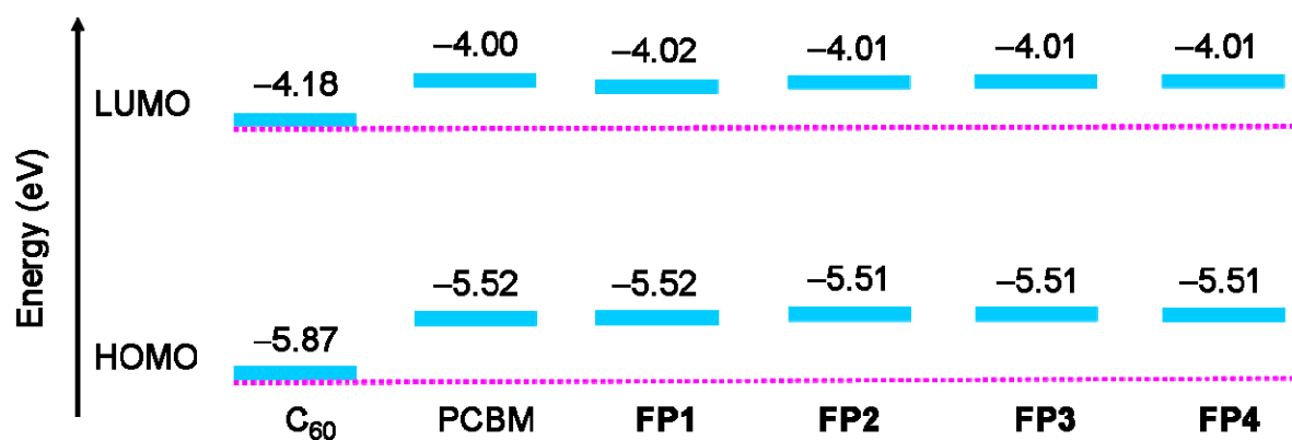
Figure 4. Schematic diagrams of HOMO and LUMO energy levels of C 60 , PCBM, and fulleropyrrolidine derivatives FP1–FP4 calculated at PBEPBE/6-311G(d, p) level.
