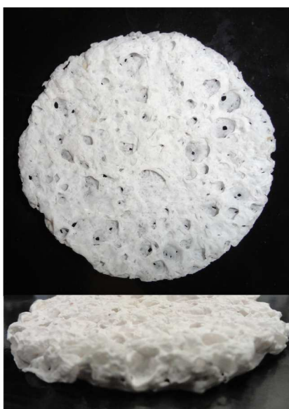
Fig. 2 Top and side view of a 54 % CB[6]-PU sponge.
