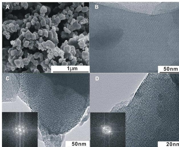
**Fig.2** (A) SEM of L-Phe-COMS; (B) TEM of template-unremoved COMS; (C) TEM of L-Phe-COMS and FFT (parallel to the pore channels) and (D) TEM of calcination L-Phe-COMS (perpendicular to the pore channels).
