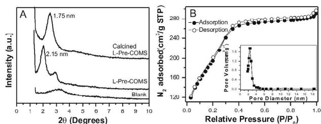
**Fig.1** (A) Low-angle XRD patterns of blank (without L-phenylalanine), L-Phe-COMS and calcined L-Pre-COMS and (B) N<sub>2</sub> adsorption-desorption isotherms of calcined L-Phe-COMS and the inset is corresponding BJH pore size distribution.
