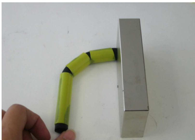
Fig. 24. Concentration graded ferrogel, the concentrations are 25, 15 and 3 wt% of iron oxide in the three regions; the highest concentration is closest to the magnet. Reproduced from ref. 84 with permission.
