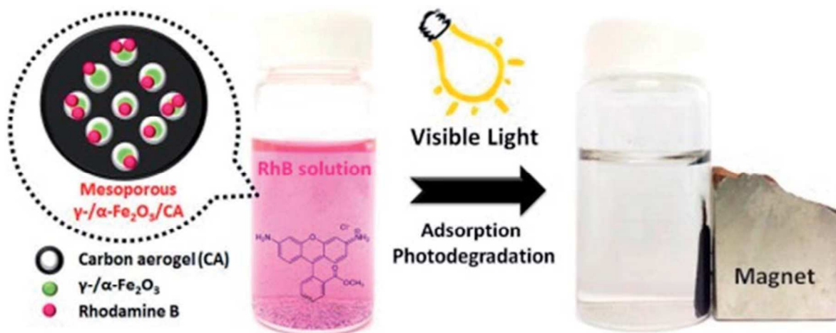
Fig. 5. Scheme of RhB dye removal using the as-prepared trifunctional \gamma - \text{Fe}_2\text{O}_3 / \alpha - \text{Fe}_2\text{O}_3 /CA structures under visible light irradiation. The tri-functional materials can be separated with an external magnetic field. Reproduced from ref. 33 with permission.
