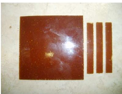
**Figure 16. Tested epoxy samples containing BAPPO particle aggregates and lumps.**
