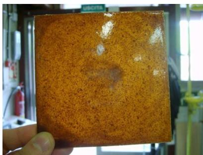
**Figure 17. Tested epoxy sample containing BAPPO particles homogeneously dispersed.**
