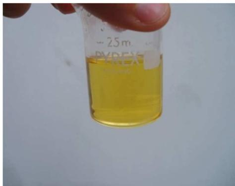
**Figure 4. Photo of T20BD+5%ECPOSS mixture after ultrasonication and 1h in a stirred oil bath at 120°C.**
