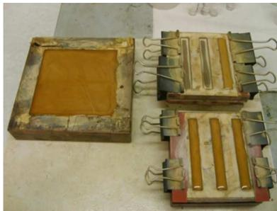
**Figure 13.** BAMPO based uncured epoxy mixture poured into molds used for fire testing.
