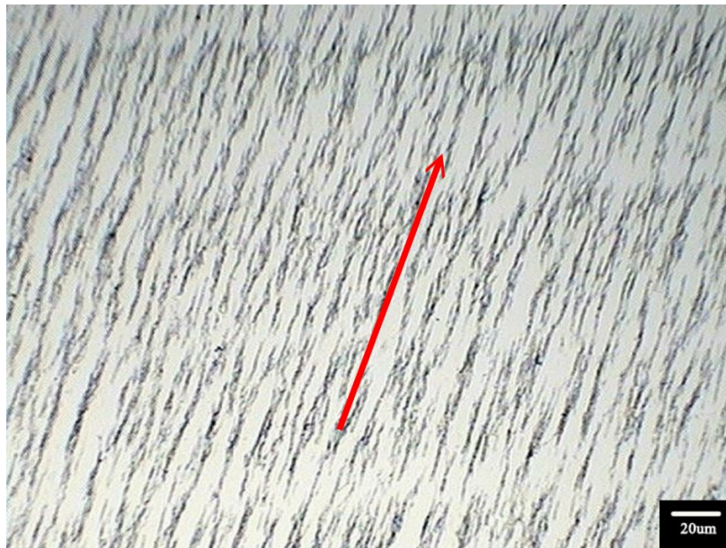
Fig.6. Photograph of the Ag-Ni nanowire alignment through an applied magnetic field.
