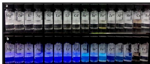
Fig. 1 Color (a) and fluorescence (b) changes of m -TAPA ( 5 \times 10^{-5} M solution in \text{CH}_3\text{CN} , 2 mL) after the addition of 200 \mu\text{L} of respective metal ions ( 5 \times 10^{-5} M solution in \text{H}_2\text{O} ).
