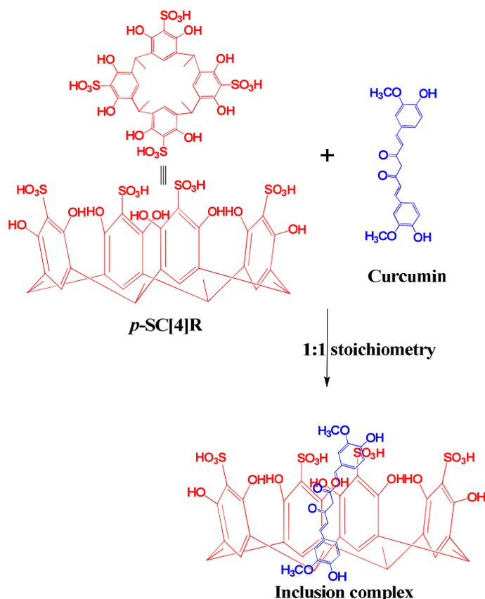
**Scheme 1** Proposed mechanism of curcumin/*p*-SC[4]R inclusion complex [1:1].
