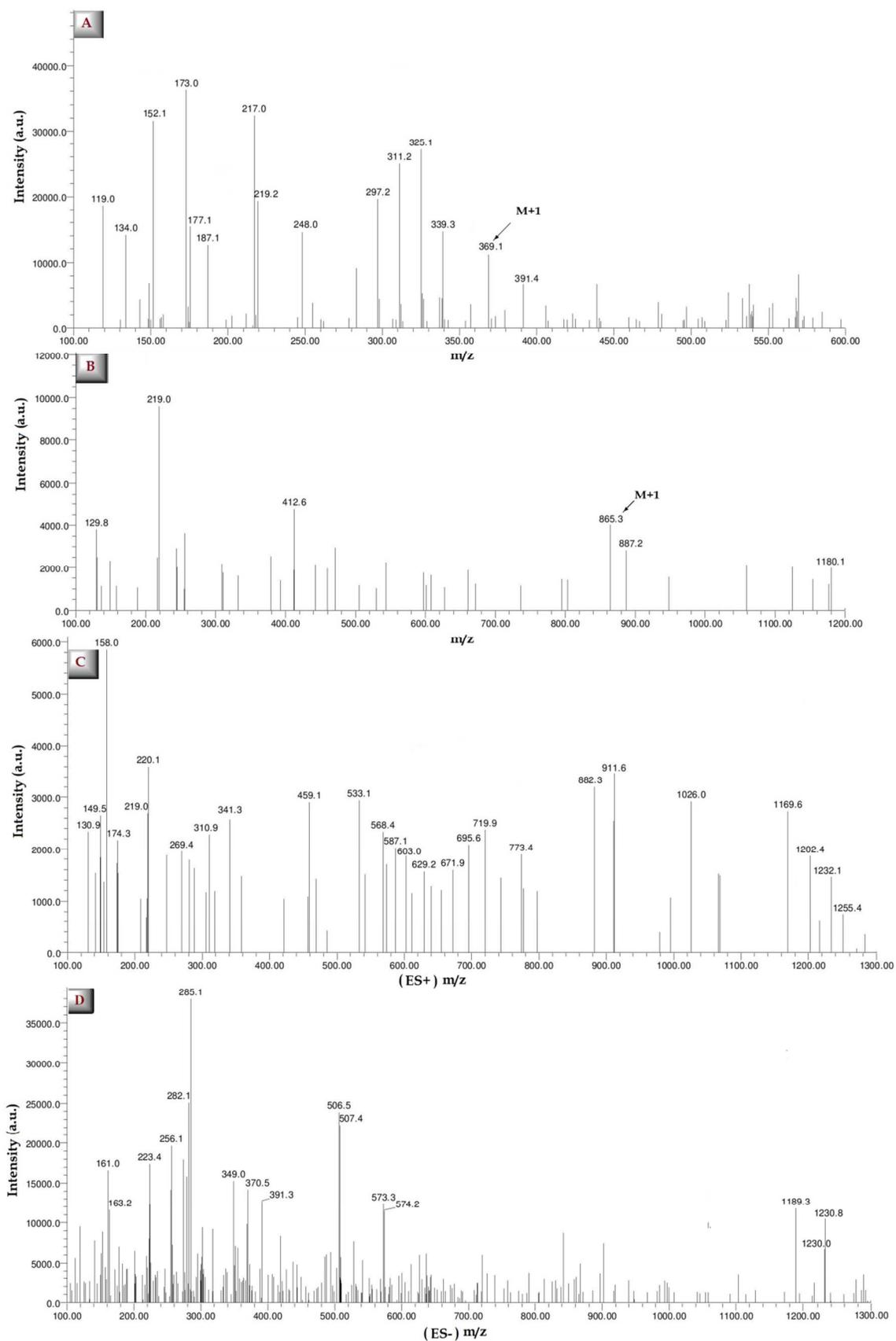
**Fig.7** ESI-MS spectra of (A) curcumin, (B) *p*-SC[4]R and (C) curcumin/*p*-SC[4]R inclusion complex (ES+ mode) as well as ES- mode spectra of inclusion complex (D).
