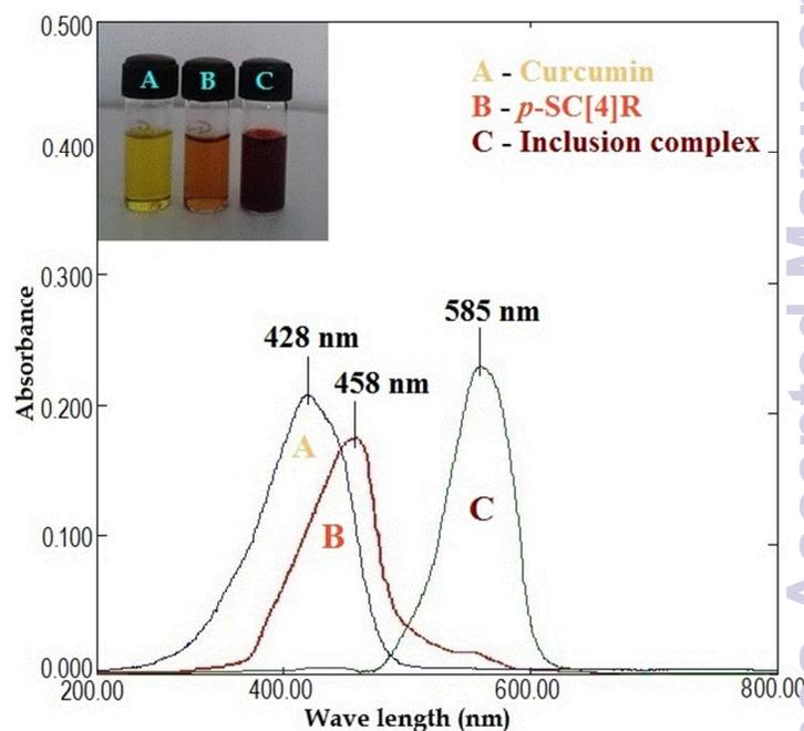
**Fig. 1** UV-Vis absorption spectra of pure curcumin, *p*-SC[4]R and inclusion complex in H<sub>2</sub>O/EtOH (50%) with visual colour changes.
