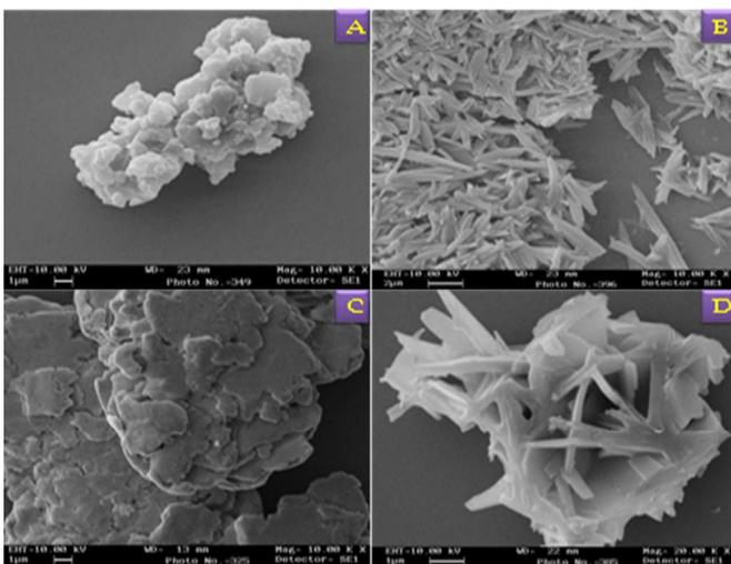
**Fig. 6** SEM micrographs of (A) Pure curcumin, (B) *p*-SC[4]R, (C) Physical mixture and (D) Inclusion complex.
