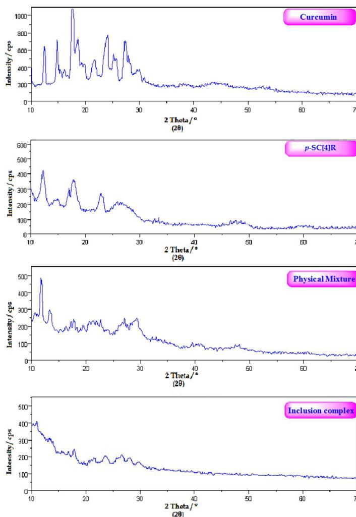
**Fig. 3** Powder x-ray diffraction patterns of curcumin, *p*-SC[4]R, physical mixture and inclusion complex.
