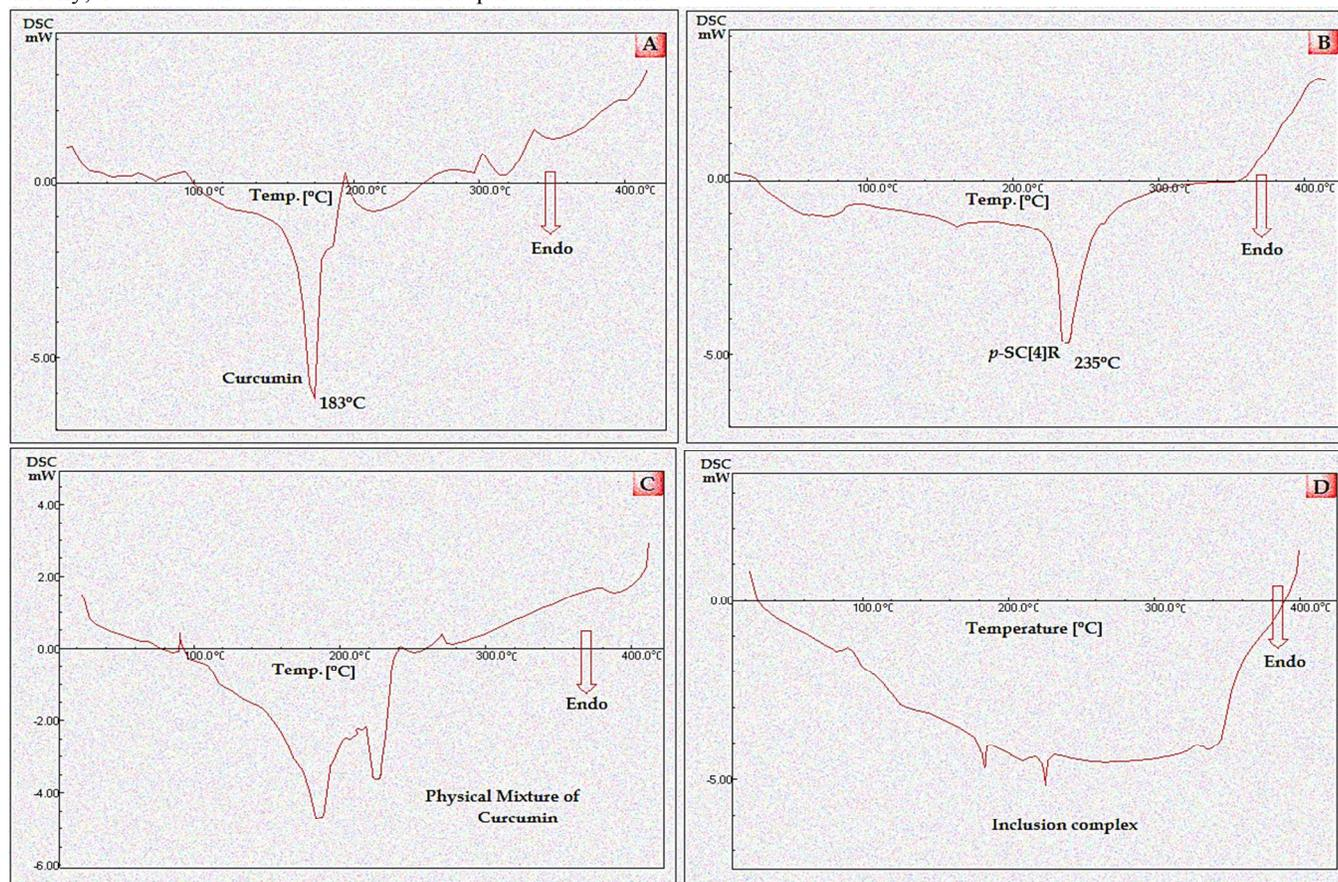
**Fig. 5** DSC thermo grams of (A) Pure curcumin, (B)  $p\text{-SC[4]R}$ , (C) Physical mixture and (D) Inclusion complex.
