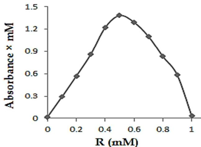
Fig. 9 Job's plot obtained for the complexation of curcumin with *p*-SC[4]R from absorption measurement at  $\lambda=428 \text{ nm}$ .
