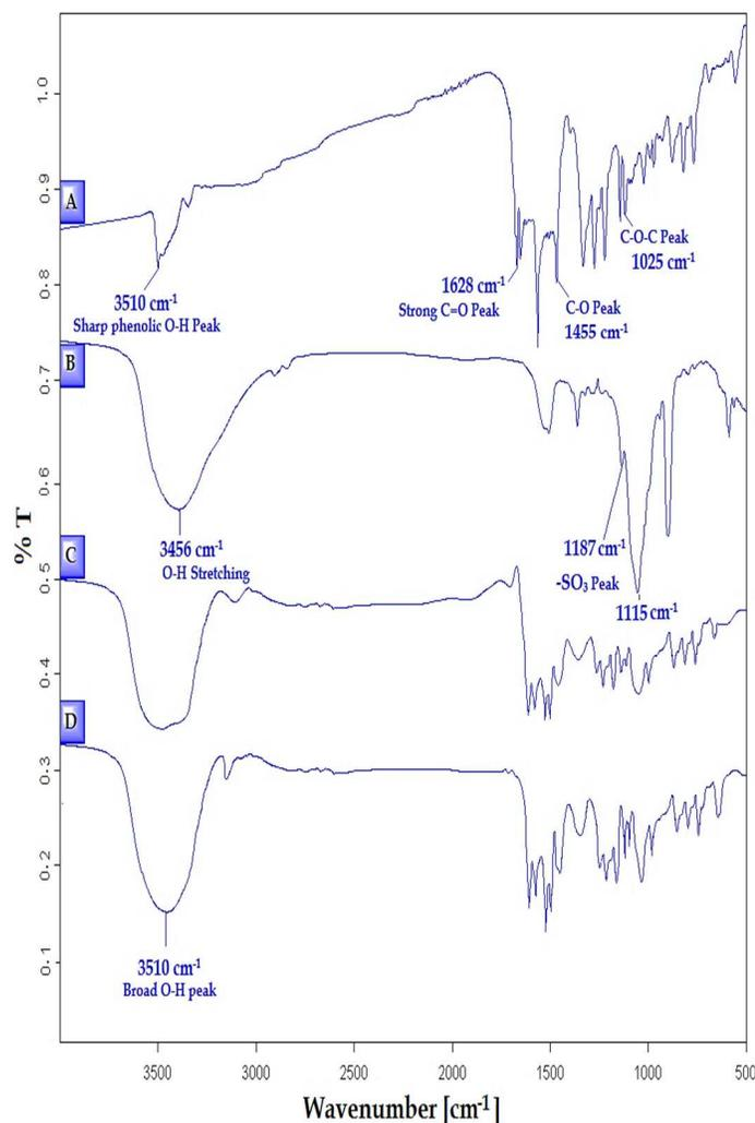
**Fig. 2** FT-IR spectra of (A) Curcumin, (B) *p*-SC[4]R, (C) Physical mixture and (D) Inclusion complex.
