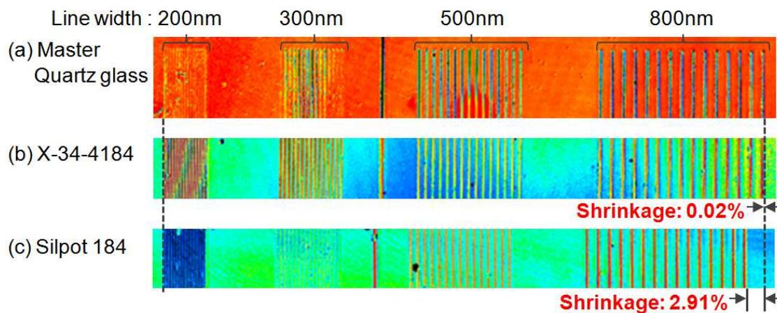
Fig. 9. Results of transfer of nanoscale line-and-space fine structure. The line groups each contain 15 lines, in line widths of 200, 300, 500, and 800 nm, all with a line:space ratio of 1:3. (a) Mold master, (b) X-34-4184, and (c) Sylpot 184.
