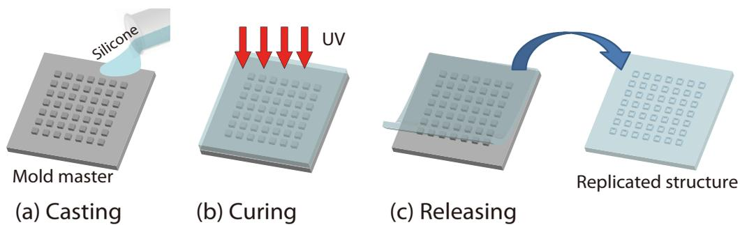
Fig. 7. Photocurable silicone elastomer replication procedure: (a) pouring the non-polymerized elastomer onto the mold, (b) exposure, and (c) peeling off.
