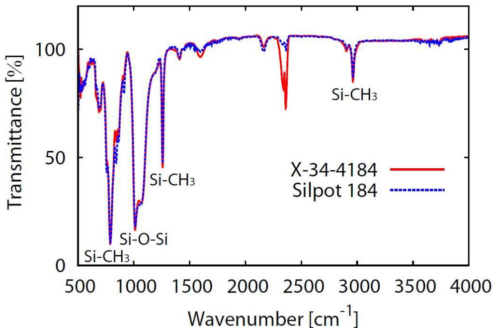
Fig. 5. Comparison of X-34-4184 and Sylpot 184 FTIR spectra. The strong peaks observable between 2280 cm<sup>-1</sup> and 2400 cm<sup>-1</sup> for X-34-4184 are presumably attributable to its photocrosslinking agent. The remainder of its spectrum is nearly identical to that of Sylpot 184, thus indicating that Sylpot 184 and X-34-4184 are nearly identical in basic molecular structure.
