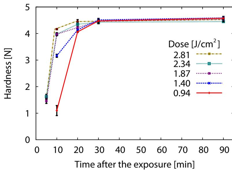
Fig. 1. X-34-4184 curing characteristics. The time course of the post-exposure curing was obtained by measurement of Shore A hardness.
