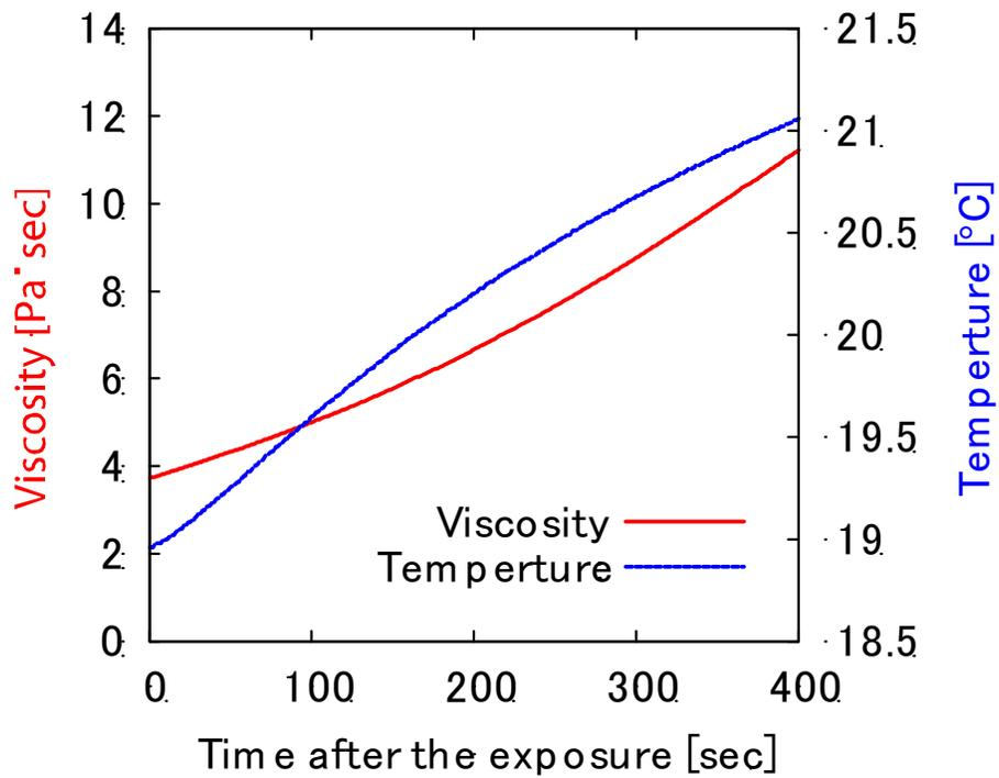
Fig. 2. Changes in viscosity and temperature of the initial post-exposure X-34-4184 in liquid form.
