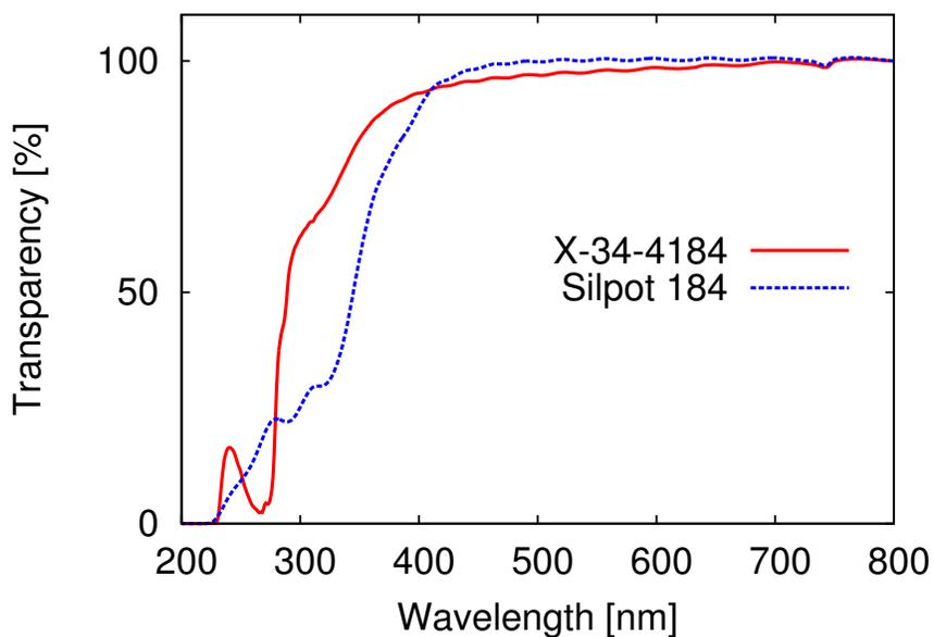
Fig. 6. Comparison of Sylpot 184 and X-34-4184 light transparency characteristics. The X-34-4184 absorption peaks around 250 nm are presumably attributable to its photocrosslinking agent. The remainder of its spectrum is nearly identical to that of Sylpot 184, thus indicating that it will exhibit nearly the same physical properties.
