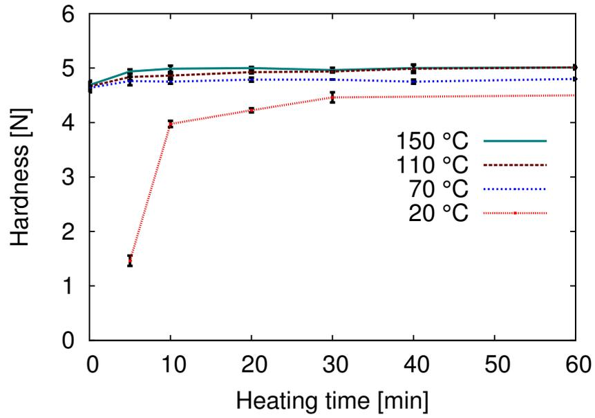
Fig. 3. Temperature dependence of X-34-4184 curing rate.
