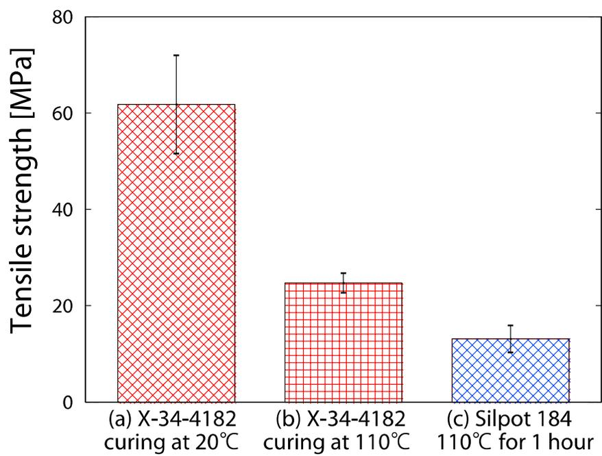
Fig. 4. Dependence of mechanical strength on curing temperature.
