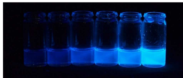
Fig. 4. The fluorescence emission of 3a in 0, 20, 40, 60, 80, and 100% DMSO (v/v) in \text{CHCl}_3 excited around 365 nm (from left). [\mathbf{3a}] = 1.25 \times 10^{-5} \text{ mol dm}^{-3} .
