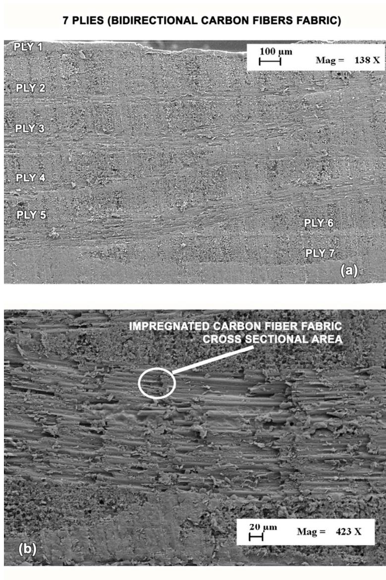
**Fig. 8.** SEM images, at two different magnification, of the cross sectional area of the manufactured panel.
