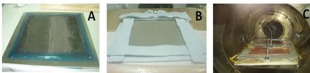
**Fig. 2.** Steps of laminate preparation.
