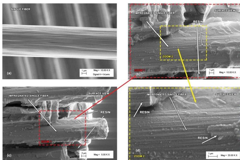
A non-usual technique to manufacture CFRCs was used. The anisotropic volumetric DC conductivity of the CFRC is almost independent on temperature in the range [30; 90] °C and is about 20 kS/m for the in plane value and 3.9 S/m for the out of plane at T=30°C. This last value is among the highest value found for CFRCs impregnated with resins loaded with carbon nanotubes and manufactured by means of a very simple process.
