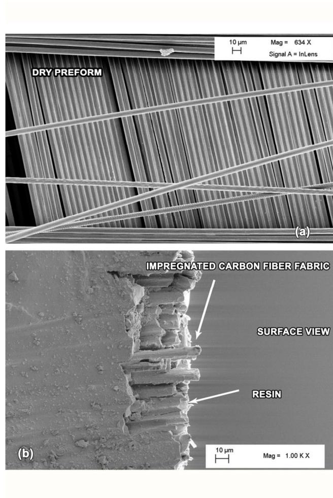
**Fig. 9.** FESEM image of the dry preform (a) and of the top side of the CFRC surface (b).
